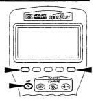
• Press the three keys shown at the same time to reset HP LogicDart.
