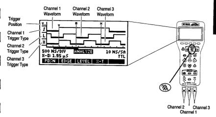
In Analyze, you have more control over waveform triggering. You can set the trigger conditions for all three channels. Press FIGSE or LEVEL to choose the trigger types, then select the channel for the trigger type using one of the CHI CHE, or CHE menu keys. The trigger position and trigger types are described on page 12.
