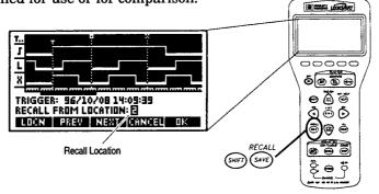
• There are 10 waveform storage locations, numbered from 1 to 10. Press NEXT or FREW to select a storage location. When the desired location is selected, press to recall the waveform and setup.
