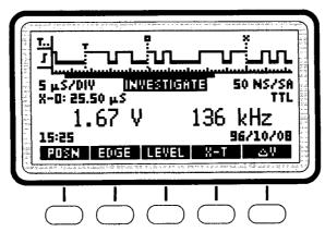
Press the menu key below the label to perform that action. In the display above, pressing the right hand menu key, labeled turns on or off the  $\Delta V$  measurement (described on page 10).
