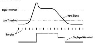
• A tolerance band exists below the high threshold and above the low threshold. An input signal value within a tolerance band can be displayed as either a logic level or a tristate level. For example, if an input signal level is in the high tolerance band, the logic level in the waveform can be either a high level or a tristate level. The width of the tolerance band depends upon the logic family used and is defined in the specifications on page 35.
