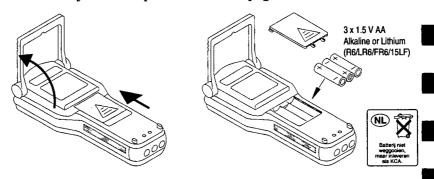
HP LogicDart calibration is not affected by dead batteries or the battery replacement procedure.
