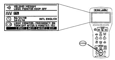
To use System Setup, move the highlight (white text on a black background) to the area of interest and then change the values for that setting. The Logic Family setting, TTL, is highlighted in the screen above.
