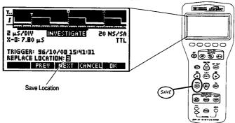
• There are 10 waveform storage locations, numbered from 1 to 10. Press NEXT or PREV to select a storage location.
