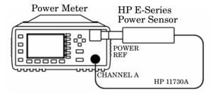
Figure 2-4: Sensor Functional Test Setup
