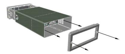
When replacing the power meter cover retighten the captive screws in the rear bezel using a 9 lb/in T15 screw driver.
