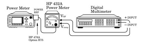
Figure 3-3: Adjustment Setup
