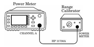
Figure 2-2: Instrument Accuracy Test Setup
