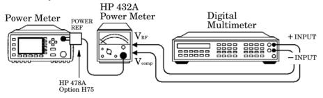
Figure 2-3: Power Reference Level Test Setup
