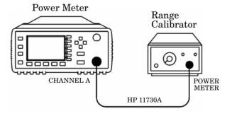
Figure 2-1: Zero Test Setup
