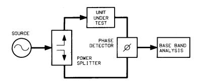
Figure 8-3 Setup for Typical Residual Phase Noise Measurement
