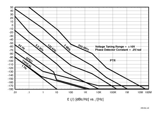
The graph shown above illustrates the equivalent phase noise at the Peak Tuning Range entered for the source due to the inherent noise at the test set Tune Voltage Output port. (A Tune Range of VCO +/-10 V and phase Detector Constant of 0.2V/Rad is assumed.)
