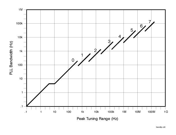
The graph shown above illustrates the closed Phase Lock Loop Bandwidth (PLL BW) chosen by the test system as a function of the Peak Tuning Range of the source. Knowing the approximate closed PLL BW allows you to verify that there is sufficient bandwidth on the tuning port and that sufficient source isolation is present to prevent injection locking.
