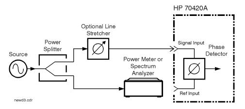
Figure 8-10 Measuring Power from Splitter
