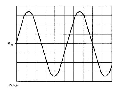
Figure 7-22 Oscilloscope Display of a Beatnote out of the Agilent/HP 70420A Monitor Port
