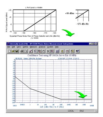
Figure 7-7 Noise Floor Calculation Example
