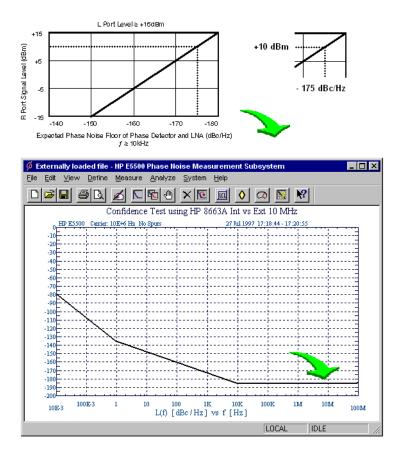
If the output amplitude of your UUT is not sufficient to provide an adequate measurement noise floor, it will be necessary to insert a low noise amplifier between the UUT and the Agilent/HP 70420A input. (Refer to "Inserting an Device" in Chapter 6, "Absolute Measurement Fundamentals" for details on determining the effect that the amplifier's noise will have on the measured noise floor.)
