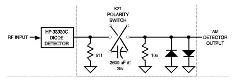
Figure 12-5 AM Detector Schematic
