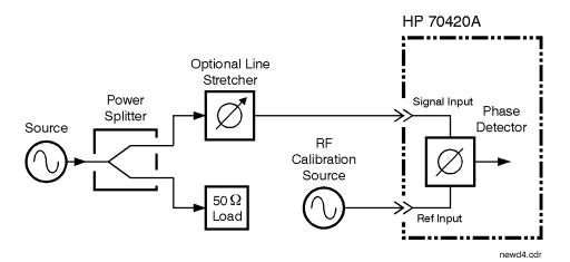
Figure 8-11 Calibration Source Beatnote Injection
