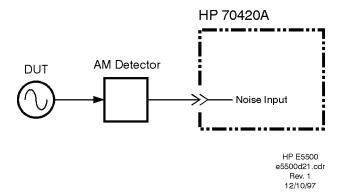
Figure 12-14 Double-sided Spur AM Noise Measurement Setup Method 1, Example 2
