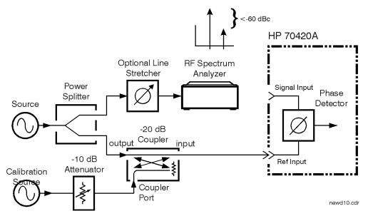
Figure 8-17 Carrier-to-spur Ratio of Non-modulated Signal
