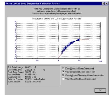
Figure 16-1 PLL Suppression Verification Graph
