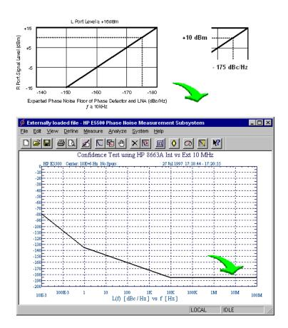
Figure 7-12 Noise Floor Calculation Example
