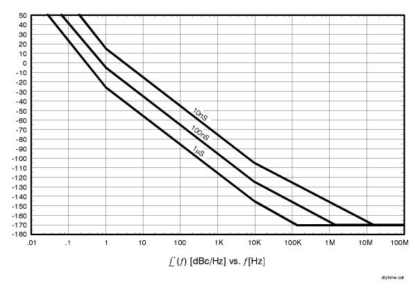
Figure 11-4 Discriminator Noise Floor as a Function of Delay Time
