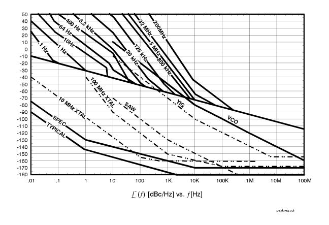
The graph shown above provides a comparison between the typical phase noise level of a variety of sources and the minimum tuning range that is necessary for the test system to create a phase lock loop of sufficient bandwidth to make the measurement. Sources with higher phase noise require a wider Peak Tuning Range.
