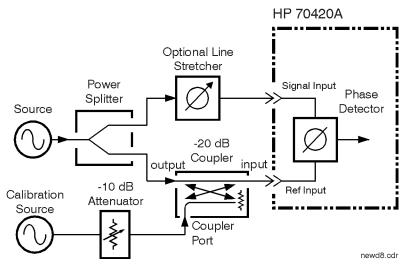
Figure 8-16 Carrier-to-spur Ratio of Modulated Signal
