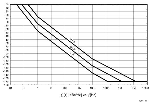
Figure 11-1 Discriminator Noise Floor as a Function of Delay Time
