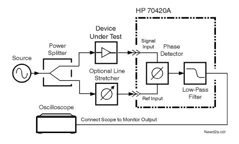
The setup for a residual phase noise measurement uses a phase shifter to set quadrature at the phase detector.
