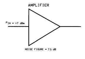
$\mathcal{L}(f) = -174 \ dBm + 7.5 \ dB - (+7 \ dBm) - 3 \ dB$  $\mathcal{L}(f) = -176.5 \ dBc/Hz$
