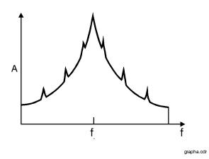
Figure 4-1 RF Sideband Spectrum
