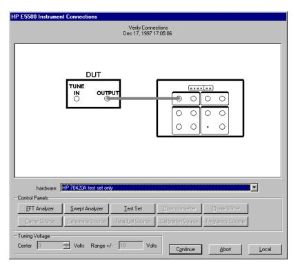
Figure 13-1 Connect Diagram for the AM Noise Measurement
