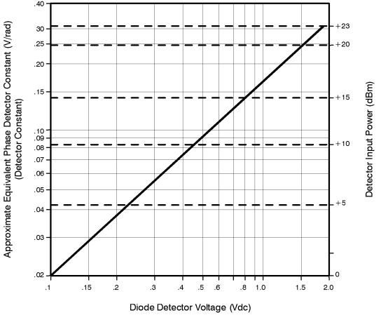
Equivalent Phase Detector Constant vs. Detector Voltage vs. Input Power
