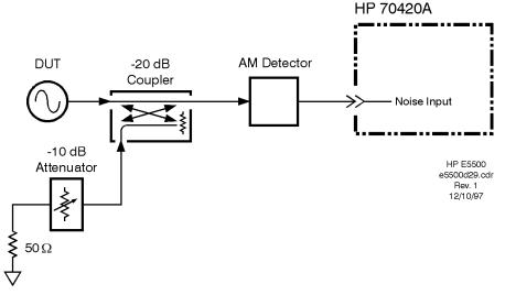
Figure 12-18 AM Noise Measurement Setup Using Single-Sided-Spur
