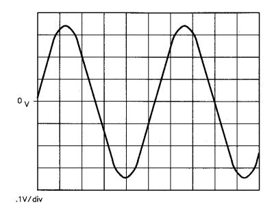
Figure 7-18 Oscilloscope Display of a Beatnote out of the Agilent/HP 70420A Monitor Port
