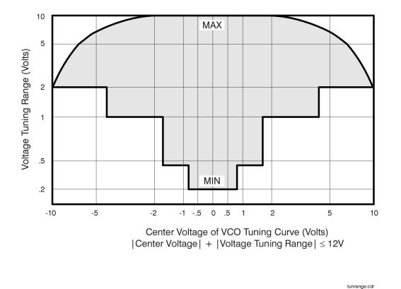
Figure 6-7 Agilent/HP 70420A Voltage Tuning Range Limits Relative to Center Voltage of the VCO Tuning Curve.
