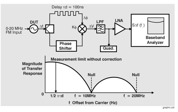
Figure 10-2 Nulls in sensitivity of delay line discriminator.
