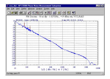
Figure 11-6 Typical Phase Noise Curve using Rate and Deviation Calibration.
