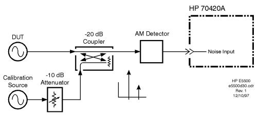
Figure 12-20 Measuring Detector Sensitivity
