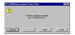
2. First establish quadrature by adjusting the phase shifter until the meter indicates 0 volts, then press Continue.
