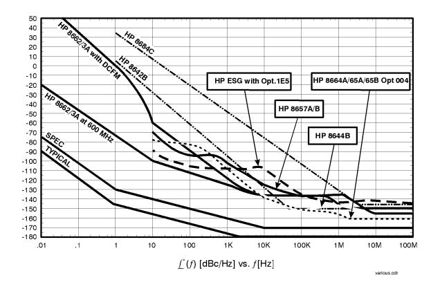
The graph shown above indicates the level of phase noise that has been measured for several potential reference sources at specific frequencies. Depending on the sensitivity that is required at the offset to be measured, a single reference source may suffice or several different references may be needed to achieve the necessary sensitivity at different offsets. Increase in Measured Noise as Ref Source Approaches UUT Noise
