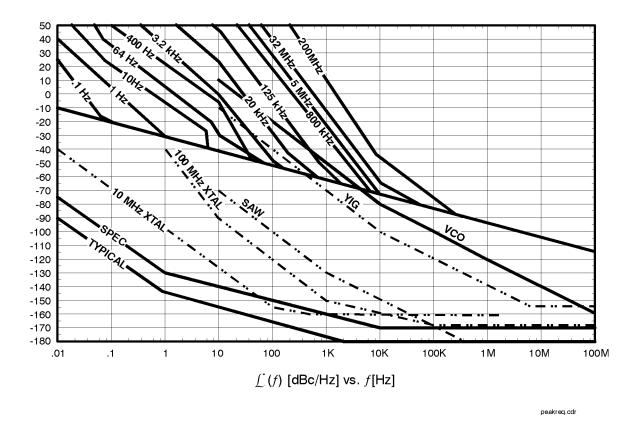
Figure 6-13 Graph Showing Peak Tuning Range Requirements for Noise that Exceeds the Small Angle Limit
