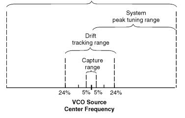
Figure 6-2 Typical Relationship of Capture Range and Drift Tracking Range to Tuning Range of VCO
