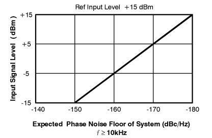
Figure 6-9 Measurement Noise Floor Relative to R Port Signal Level.
