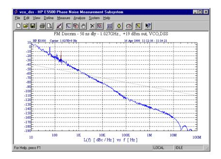
Figure 11-3 Typical Phase Noise Curve using Double-Sided Spur Calibration.
