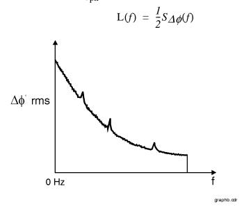
Figure 4-2 CW Signal Sidebands viewed in the frequency domain
