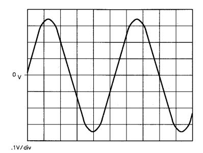
Figure 7-4 Oscilloscope Display of a Beatnote out of the Agilent/HP 70420A Monitor Port
