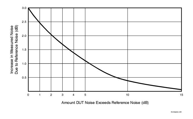
The graph shown above demonstrates that as the noise level of the reference source approaches the noise level of the UUT, the level measured by the software (which is the sum of all sources affecting the test system) is increased above the actual noise level of the UUT.
