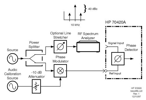
Figure 8-14 Measuring Carrier-to-sideband Ratio of the Modulated Port
