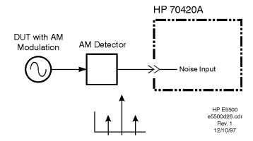
Figure 12-13 Measuring the Calibration Constant
