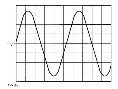
Figure 5-4 Oscilloscope Display of a Beatnote out of the Agilent/HP 70420A Monitor Port
