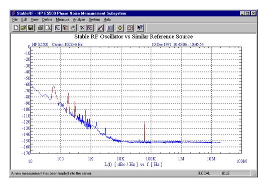
Figure 7-5 Typical Phase Noise Curve for a Stable RF Oscillator.
