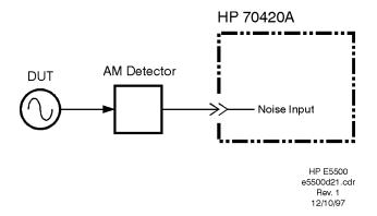
Figure 12-9 User Entry of Phase Detector Constant AM Noise Measurement Setup Method 1, Example 2
