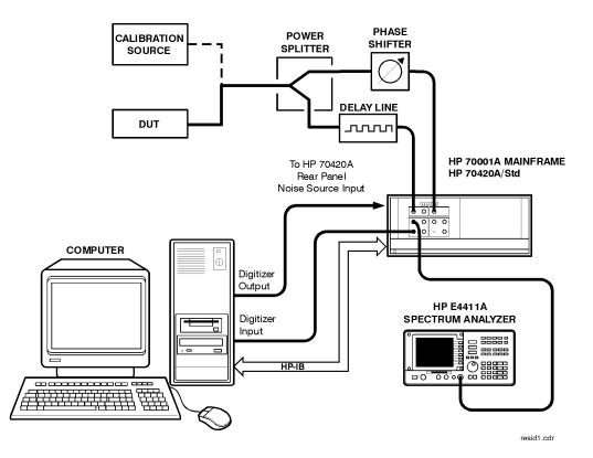
4. The system can now run the measurement. at the appropriate point, re-establish quadrature and continue the measurement.
