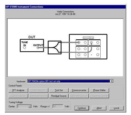
*Figure 9-1* Setup diagram for the Agilent/HP 8349A Amplifier Measurement Example.
