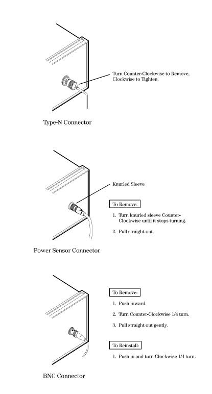
Figure A-2 Type-N, Power Sensor, and BNC Connectors
