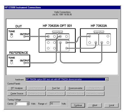
Figure 7-21 Connect Diagram for the Microwave Source Measurement
