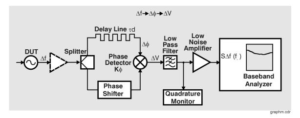
In the Discriminator measurement, the source is placed ahead of the power splitter. One output of the splitter feeds a delay line with enough delay to decorrelate the source noise. The delay line generates a phase shift proportional to the frequency. The phase shift is measured in the phase detector by comparing the delay output with the other output from the splitter. The output of the phase detector is a voltage proportional to the frequency fluctuations of the source.
