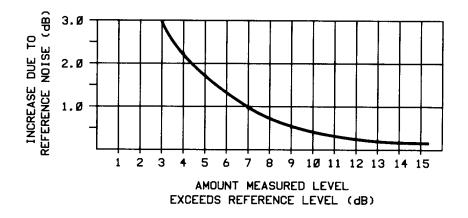
Figure 15-3 Graph Showing How Much to Decrease Measured Noise to Compensate for Added Reference Source Noise.
