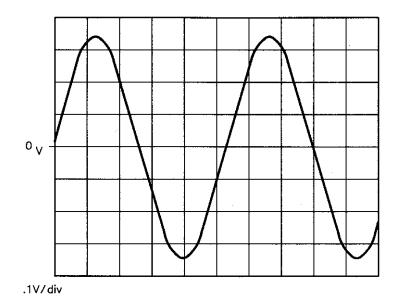
Figure 5-9 Oscilloscope Display of a Beatnote out of the Agilent/HP 70420A Monitor Port
