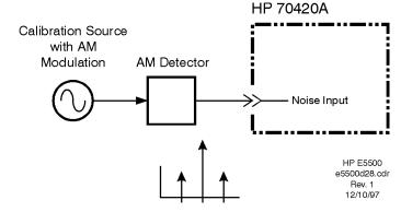
Figure 12-17 Measuring the Calibration Constant
