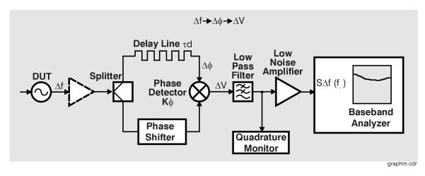
Figure 10-1 Basic delay line/mixer frequency discriminator method.
