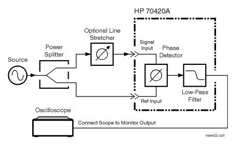
Figure 8-9 Connection to Optional Oscilloscope for Determining Voltage Peaks
