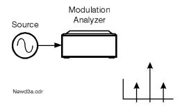
Figure 12-12 Measuring the Carrier-to-Sideband Ratio
