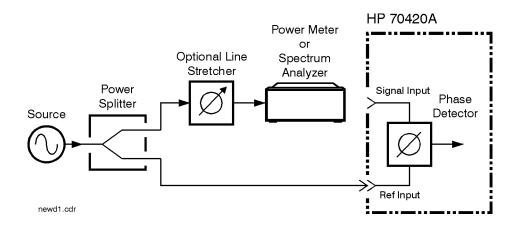
Figure 8-6 Measuring Power at Phase Detector Signal Input Port
