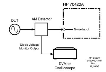
Figure 12-10 Modulation Sideband Calibration Setup
