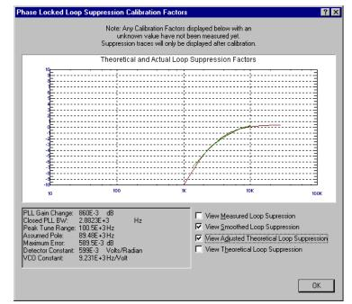
Figure 16-8 Smoothed vs Adjusted Theoretical Loop Suppression Curve
