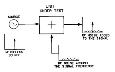
Figure 8-1 Additive Noise Components
