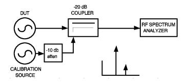
Figure 12-19 Measuring Relative Spur Level
