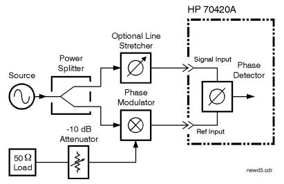
Figure 8-13 Calibration Setup
