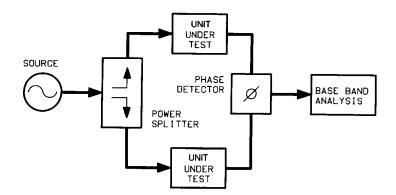
Figure 8-4 Measurement Setup for Two Similar UUTs
