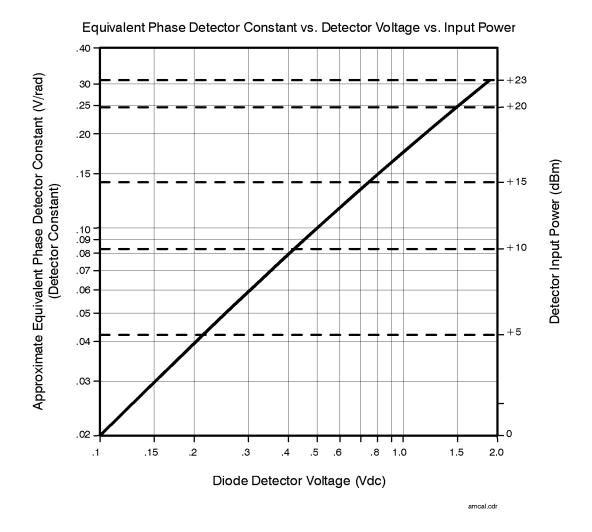
The AM detector sensitivity graph shown above is used to determine the equivalent phase Detector Constant from the measured AM Detector input level or from the diode detector's dc voltage. The equivalent phase Detector Constant (phase slope) is read from the left side of the graph while the approximate detector input power is read from the right side of the graph.
