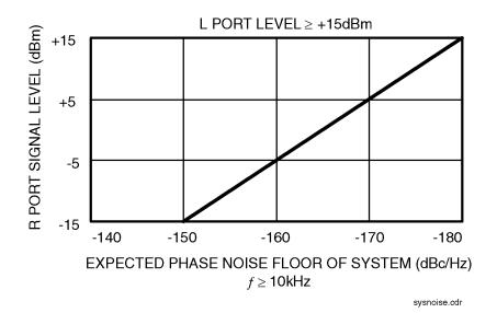
Figure 5-6 Noise Floor for the Agilent/HP 8644B 10 MHz Measurement
