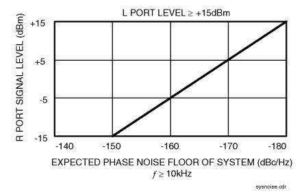
Figure 5-1 Noise Floor for the Agilent/HP 8663 10 MHz Measurement
