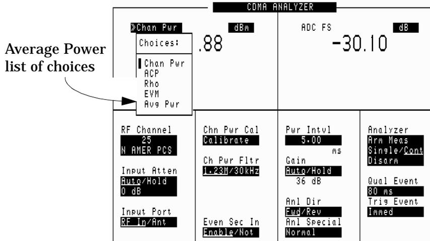
7. Set the **Pwr Intvl** to your desired averaging time. A higher time produces a more accurate result. Maximum value is 26.66 milliseconds.
