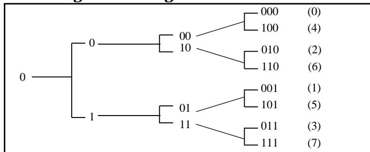
To generate a Walsh code tree, take the initial code, first add a place (bit) in the most significant number's (MSN) place. Then, for the upper branch, give this bit the value "0". Finally, for the lower branch give this number the value "1". This process proceeds to generate more and more branches until you have reached the desired Walsh code length. The code sets are denoted by their length in bits which corresponds to the
