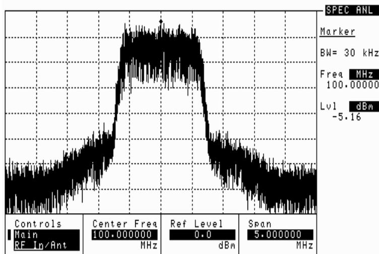
Sometimes the “Shoulders” also occur when there is an interfering signal near the CDMA signal. In this case, the “Shoulders” are usually much smaller in bandwidth.
