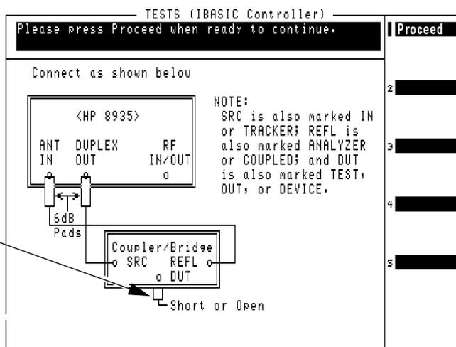
When measuring the swept return loss of a transmission line that is not terminated at an antenna, terminate the line into a 50Ω load.
