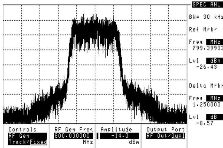
Seeing “Shoulders” on the Spectrum Analyzer display is one common distortion of the CDMA shape. This problem usually occurs when there is a problem with the power amplifier of the Base Station. The bandwidth of the “Shoulders” is usually about twice the bandwidth of the 1.2288 MHz CDMA signal.
