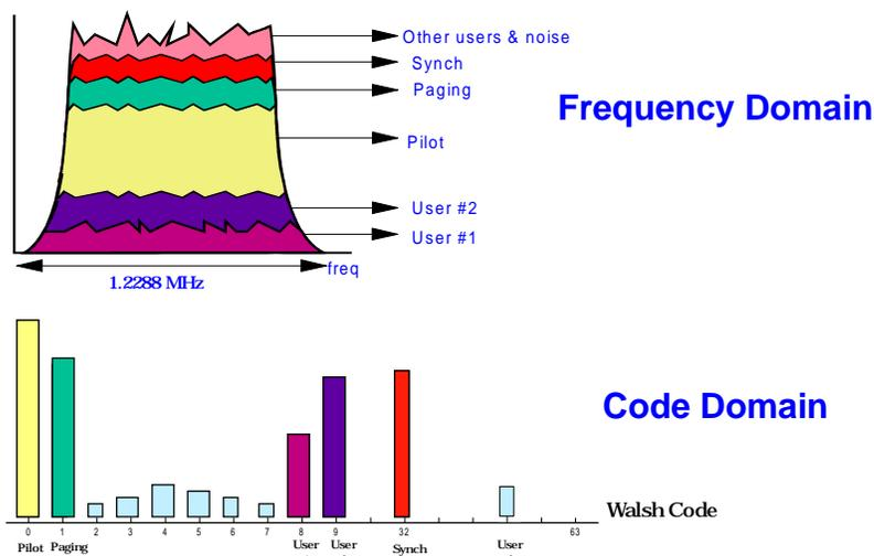
On a spectrum analyzer, you can view the 1.23 MHz forward link channel; it would appear as the envelope of the top figure. But how much of the total signal, as viewed on the spectrum analyzer, is attributed to each individual Walsh code? You cannot tell using frequency domain analysis. This, again, requires a new measurement method.
