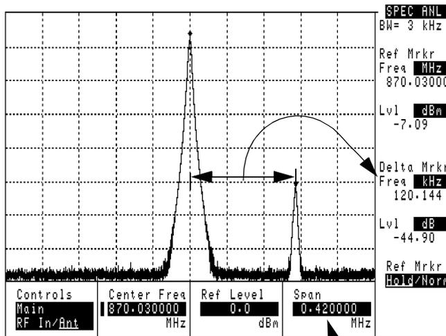
Using the Delta Markers function, you can see that a smaller signal is only 120 kHz (four channel spacings) away from the signal you want to measure. In this case, set [Parameter 31 - TX Use 230 kHz BW on Data Dev \[1=yes\]](#) to **0** to reduce the measurement bandwidth, or turn off the other radio.
