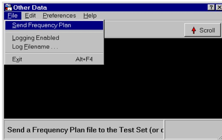
**Step 7.** Select the frequency plan file that you saved (see [Figure 2-22](#)). Double-click on the file name, or select the file name and select **Open**. The frequency plan will be downloaded to the Test Software.
