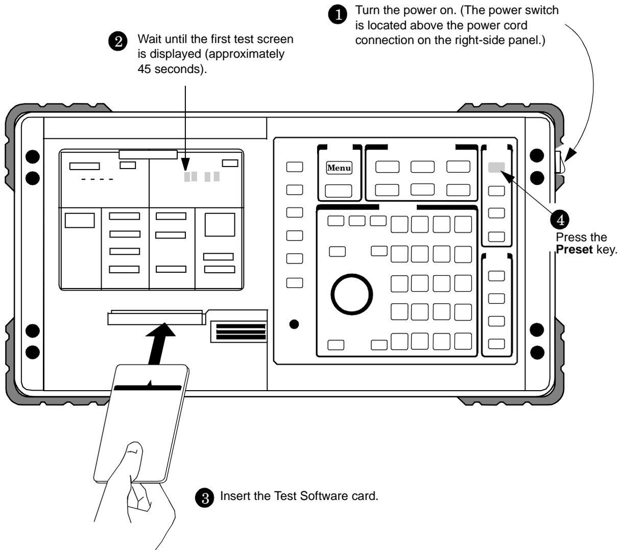
**Figure 2-2 Loading and Running the Test Software (continued)**
