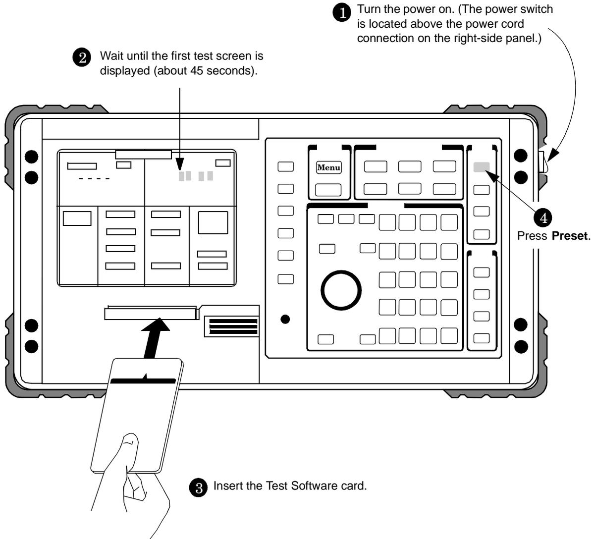
**Figure 5-4 Loading a Procedure**
