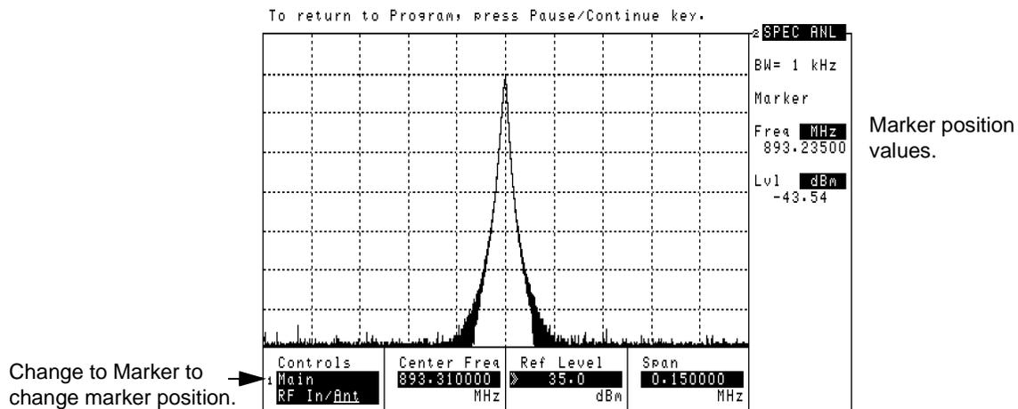
Use the **Ref Level** and **Span** fields for the best view of the transmitted signal.
