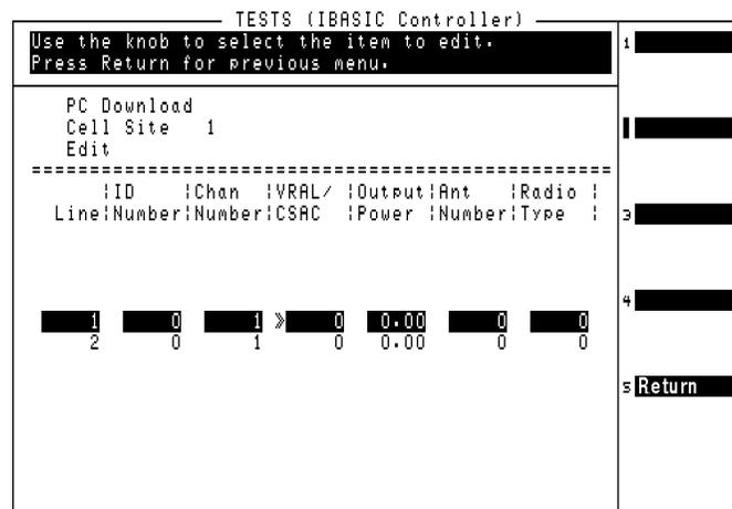
**Step 6.** Use the **Line** field to select each line in the plan (which corresponds to individual radios in the site), and then enter these values for each line:
