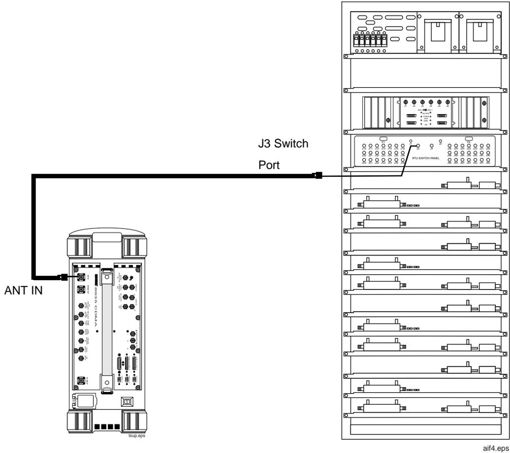
Figure 3-2 Series II Base Station TX Antenna Port (Out of Service) Connections
