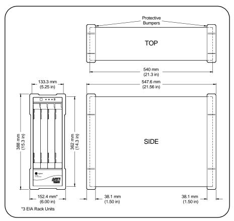
Figure A-1. E8408A Mainframe Dimensions
