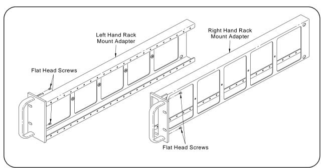
Figure 2-5. Attaching Handles to the Rack Mount Adapters
