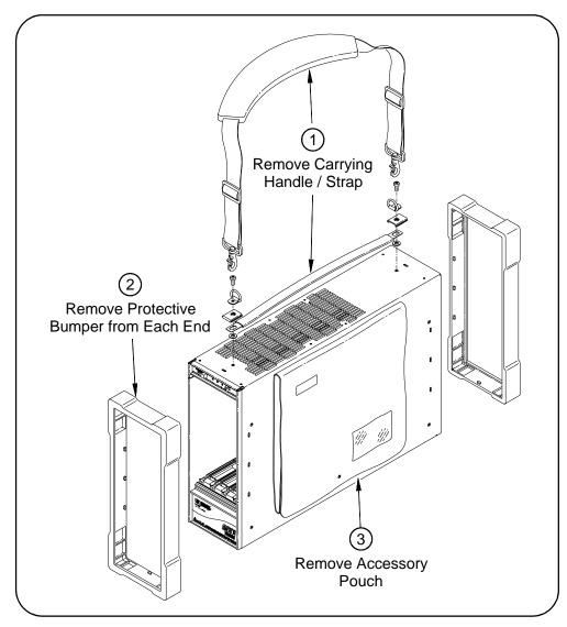
Figure 2-13. Removing Mainframe Items
