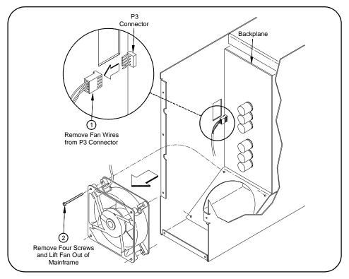
Figure 3-5. Removing the Fan Assembly
