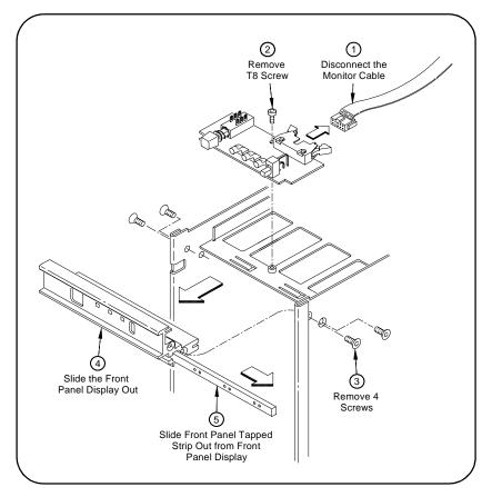
Figure 3-6. Removing the Front Panel Tapped Strip
