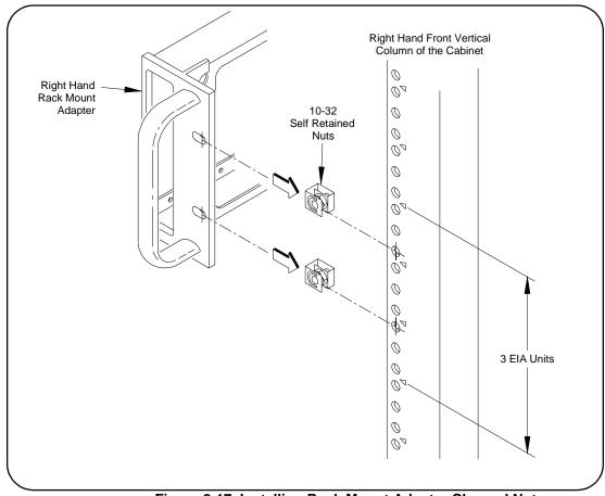
Figure 2-17. Installing Rack Mount Adapter Channel Nuts
