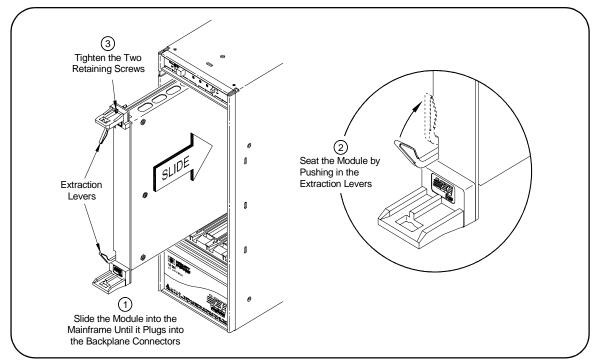
Figure 1-3. Installing C-Size Instruments in the E8408A Mainframe
