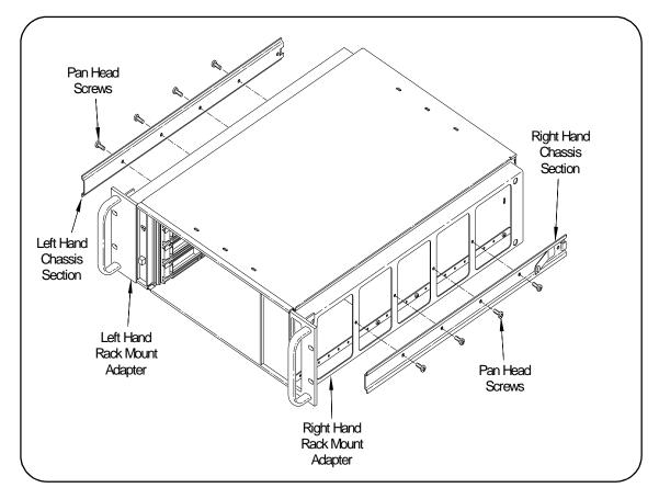
Figure 2-8. Connecting Chassis Section to Rack Mount Adapters
