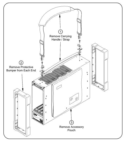
Figure 2-3. Removing Mainframe Items
