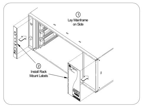
Figure 2-4. Installing Rack Mount Labels
