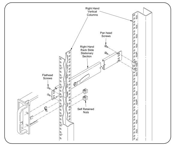
Figure 2-10. Installing Rack Slide Stationary Sections
