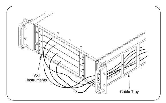
Figure 2-12. Routing VXI Instrument Cables
