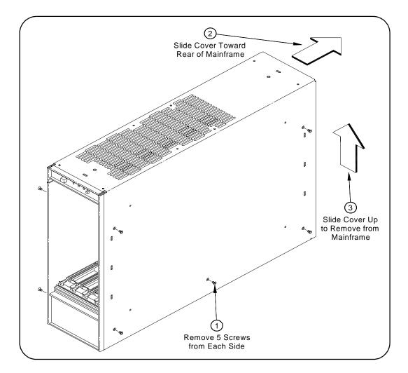
Figure 3-2. Removing the Mainframe Cover
