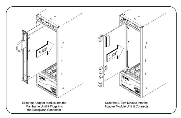
Figure 1-4. Installing A- and B-Size Instruments in the E8408A Mainframe
