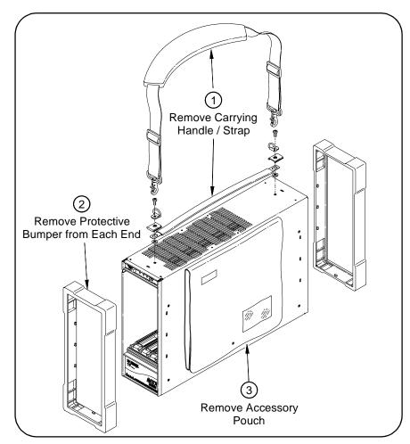
Figure 3-1. Removing Mainframe Accessory Items
