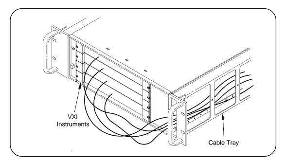
Figure 2-20. Routing VXI Instrument Cables
