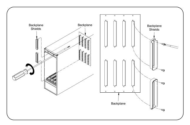
Figure 2-22. Positioning the Backplane Shields on the Connectors.
