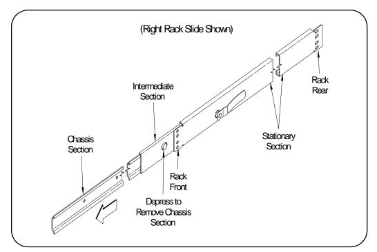
Figure 2-7. Removing Rack Slide Chassis Section
