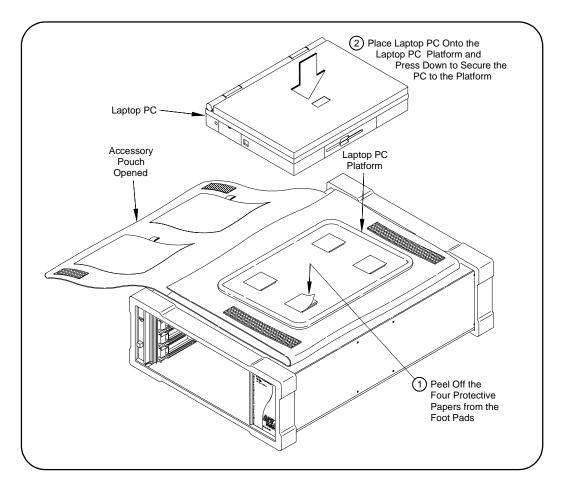
Figure 2-2. Attaching Laptop PC to Accessory Pouch
