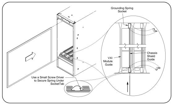
Figure 2-21. Installing the Grounding Springs and Chassis Shield.
