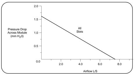
Figure A-2. E8408A Mainframe Cooling Capacity
