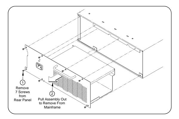
Figure 3-3. Removing the Power Supply Assembly
