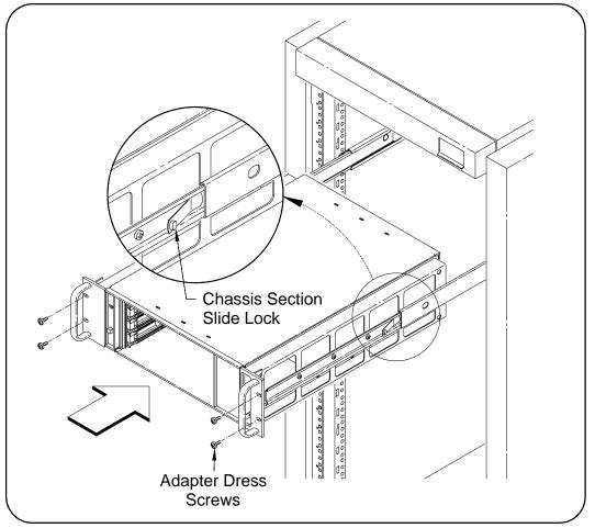
Figure 2-11. Installing the Mainframe
