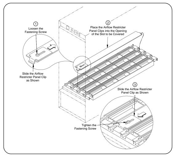
Figure 2-23. Installing the Airflow Restricter
