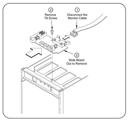
Figure 3-4. Removing the Monitor Board
