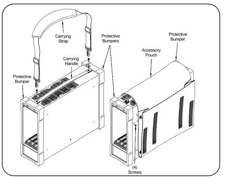
Figure 2-1. Attaching Carrying Strap and Accessory Pouch
