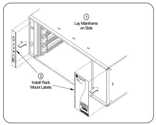
Figure 2-14. Installing Rack Mount Labels
