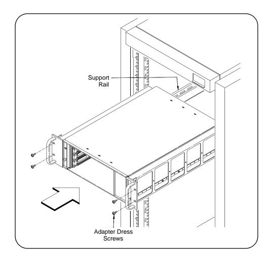
Figure 2-19. Installing the Mainframe
