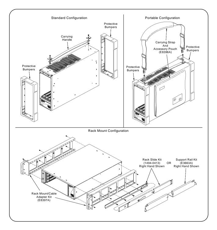
Figure 1-1. E8408A Mainframe Configurations/Options
