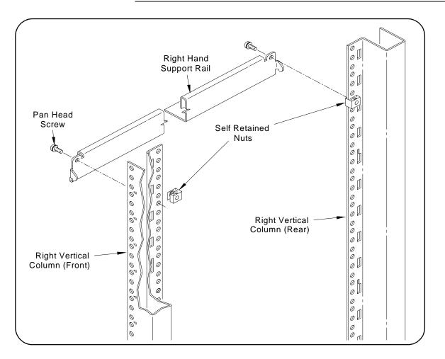
Figure 2-18. Installing Support Rails
