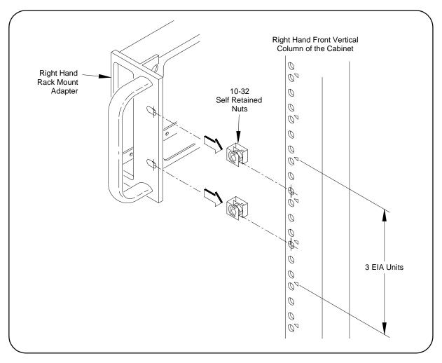
Figure 2-9. Installing Rack Mount Adapter Channel Nuts
