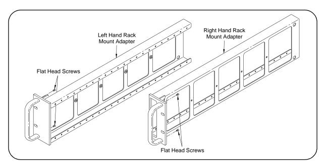
Figure 2-15. Attaching Handles to the Rack Mount Adapters
