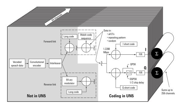
Physical layer of CDMA standard block diagram.
