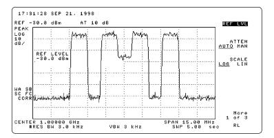
Multicarrier spectrum corresponding to the custom configuration.
