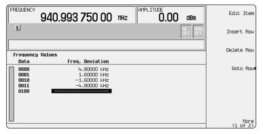
You can build asymmetric FSK formats such as FLEX with the FSK table editor.
