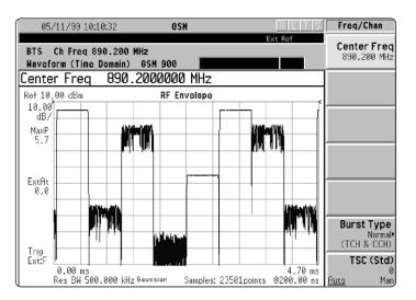
Synchronize two ESGs to combine EDGE (8PSK) and GSM (GMSK) timeslots.
