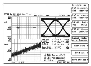
89441A display of modulation quality of a Bluetooth signal generated by an ESG.
