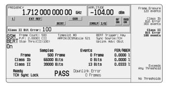
GSM base station bit error rate test.
