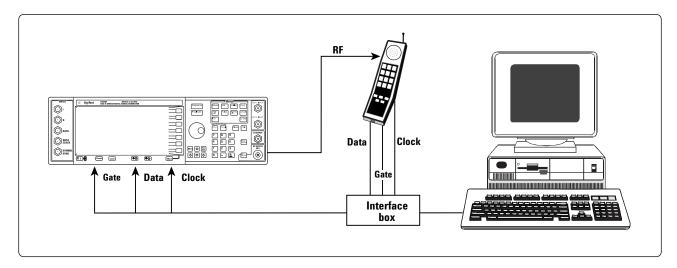
Common setup for bit-error-rate measurement of mobile phones.
