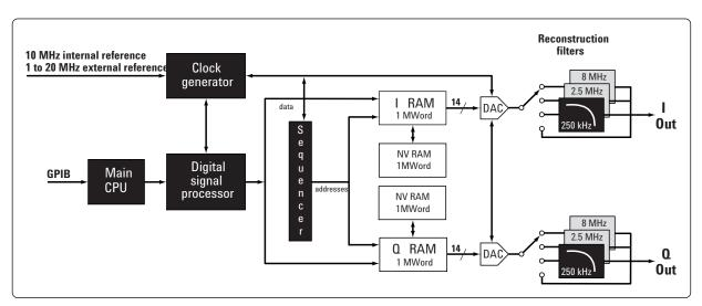
High-performance internal dual arbitrary waveform generator block diagram.
