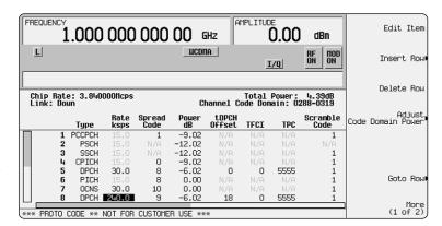
Use the flexible table editor to fully configure a W-CDMA signal waveform.
