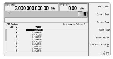
FIR table allows custom modulation filtering.
