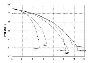
Peak/average cumulative distribution function of IS-95 waveforms.
