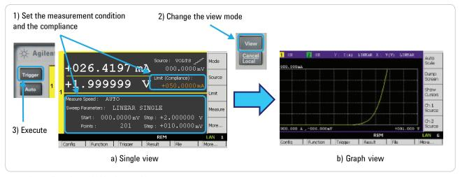
Figure 3. The GUI of the B2900A Series of SMUs makes it easy to take a quick measurement and display the results
