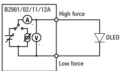
Figure 1. Example of OLED characterization using the B2900A Series of SMUs
