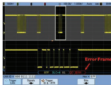
Turning on serial decode on Agilent's InfiniiVision 7000B has no impact on its waveform update rate, and it is able to capture the error frame on this CAN bus
