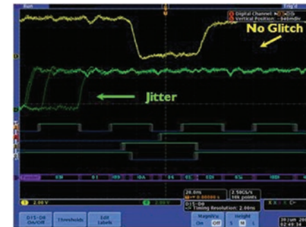
Tektronix MDO4000 Series update rate drops when you turn on deep memory and digital channels, and the scope misses the signal jitter and metastable state
