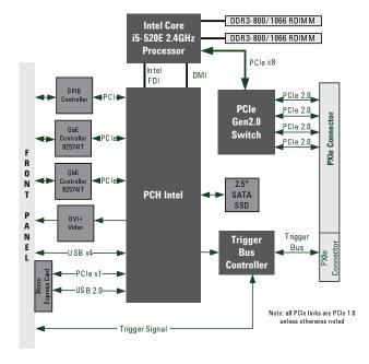
Figure 2. M9036A block diagram
