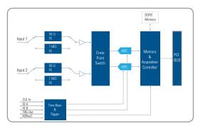
Figure 2. Simplified block diagram of the M9210A PXI-H Digitizing Scope.
