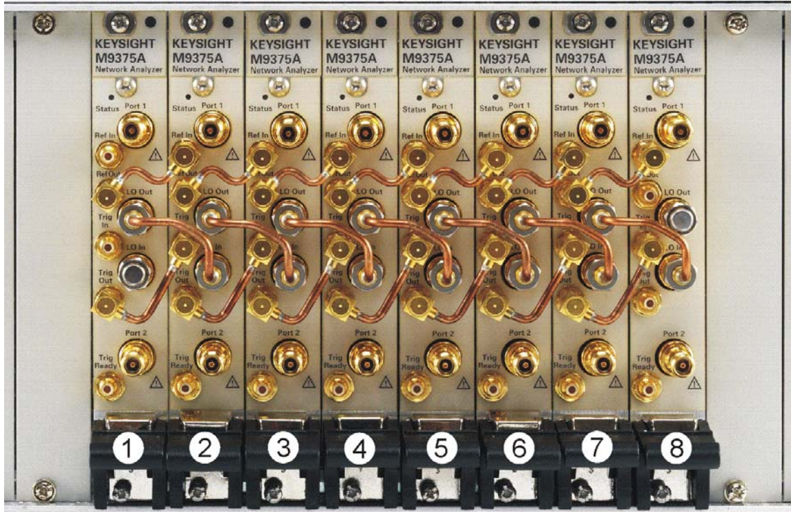
Figure 1-10 Installing Semi-Rigid Cable M9370-20019
