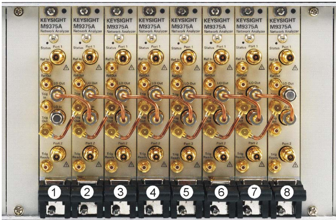
Figure 1-9 Installing Semi-Rigid Cable M9370-20006
