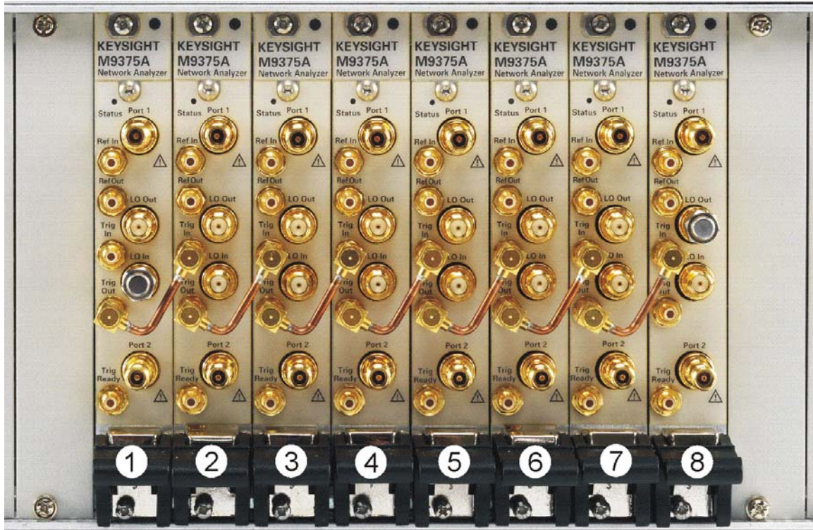
Figure 1-7 Installing Semi-Rigid Cable M9370-20018
