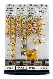
Figure 1. M9391A PXIe vector signal analyzer with four modules consisting of the M9300A frequency reference, M9301A synthesizer, the M9350A downconverter and the M9214A digitizer.
