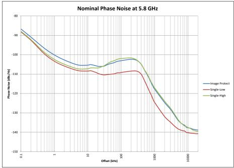
Figure 9. Phase noise at 5.8 GHz.
