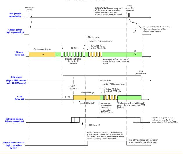
In brief, the host PC must be off whenever the chassis is powered up or down. Because modules are not hot-swappable, the chassis must be powered down before modules are added or removed.
