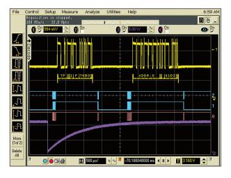
Precise MSO triggering and display Mixed-signal oscilloscope measurement in a mobile system using both digital and analog acquisition channels.
