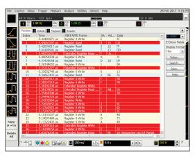
Compact protocol using the full screen listing. The protocol viewer window shows the index number, time stamp value identifier, packet type, and data values for each MIPI RFFE packet. Data in the listing window can be saved to a .csv or .txt file for offline viewing.
