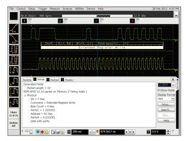
Quickly move between physical and MIPI RFFE protocol layer information using the time-correlated tracing marker. Display protocol content using embedded decode in the waveform area, or see protocol events in a compact listing format. Minor tick marks indicate clock transitions. Major tick marks indicate segments of the serial packet MIPI RFFE measurements and are automatically time-correlated with measurements on other oscilloscope channels.
