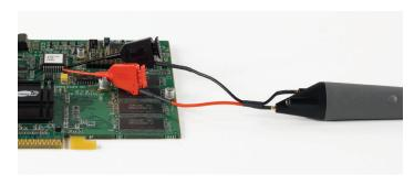
Use flex nose clip adapters with the dual lead adapter to obtain access to IC leads or head connectors.
