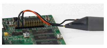
The dual lead adapter allows you to easily connect the probe to a popular 0.1" pin header with 0.025" square pins.
