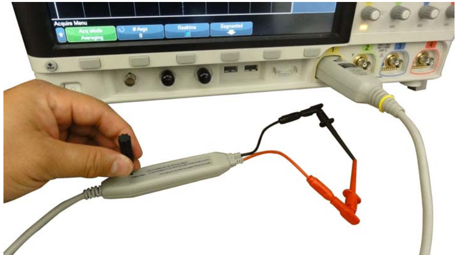
Figure 7 Adjusting the Offset Using the Supplied Tool
