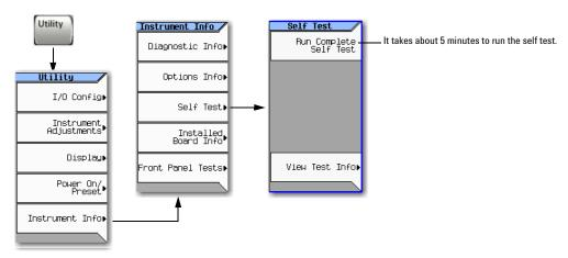
Use the following procedure to run self test:
