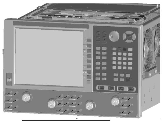
(1) Reinstall 12x jumper cables N5222-20091 and torque to 10 in-lbs.
