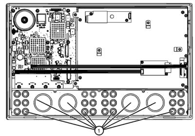
Old lower front-panel overlay visible through cutouts from rear of front panel.
