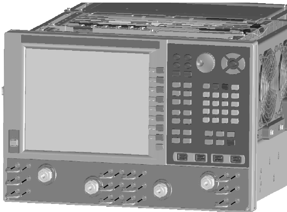
Figure 11 Front Panel Jumper Cables Installation
