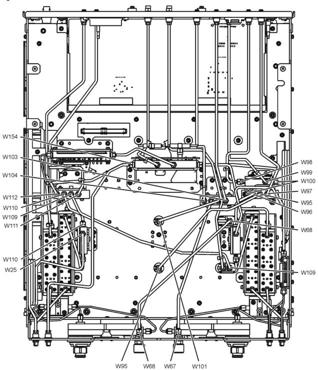
Figure 15 New Test Set Cable Installation
