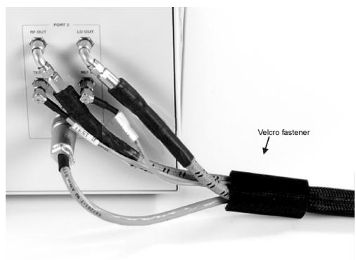
Figure 3-4 Details for Controller Front Panel Connections
