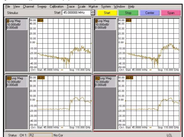
Figure 6-1 Typical Receiver Display for a 2-Port System
