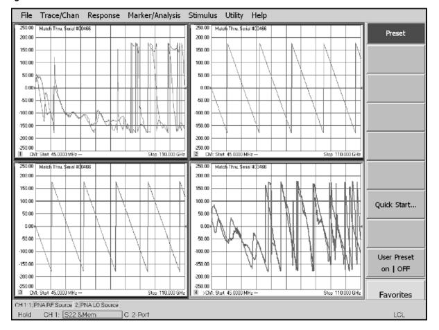
Figure 6-9 Phase for Mismatched Thru
