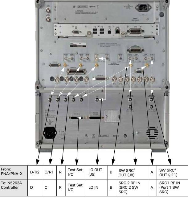
a. Install the adapters (N4903-61250) on the N5224/25A or N5244/45A SW SRC OUT (J8 and J11).
