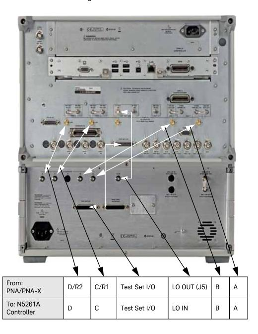
Figure 1-16 N5262A Rear Panel Configuration B
