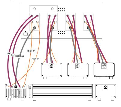
Figure 1-24 Example; VDI Module Connections
