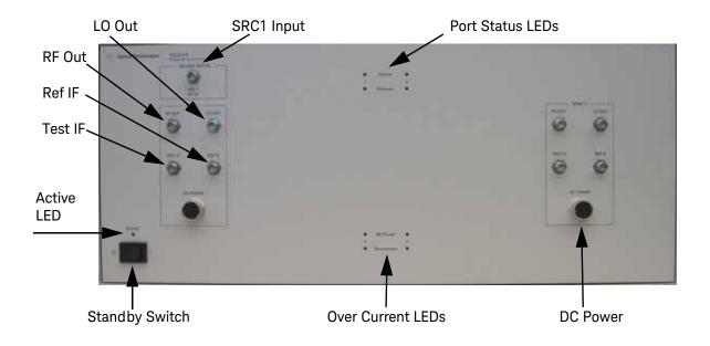
Figure 1-6 N5262A (4-Port) Front Panel Features
