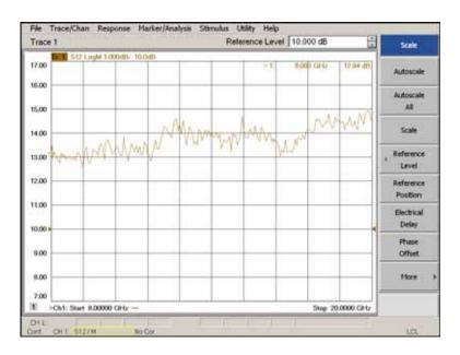
Figure 2-3 RF Output Gain with +2 dBm ALC Off
