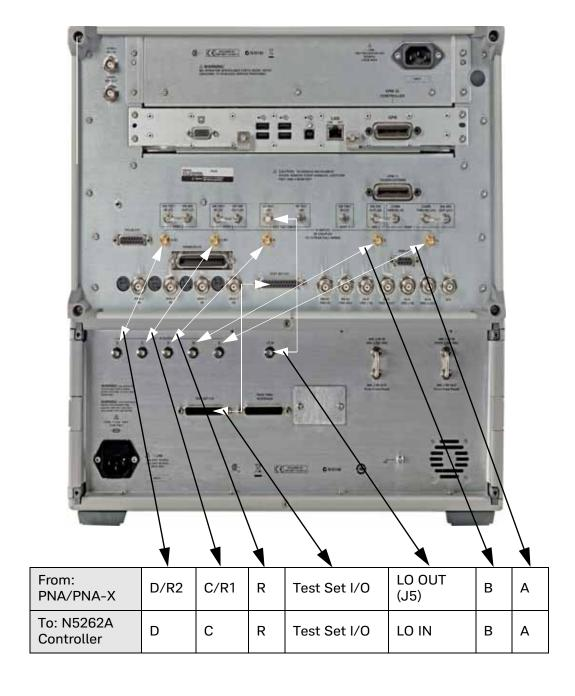
Figure 1-17 N5261A Rear Panel Configuration C
