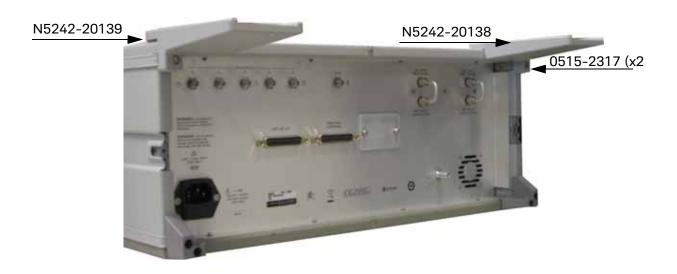
6. Place the analyzer on top of the test set and ensure that the front frame of the analyzer is positioned slightly forward of the locks that are attached to the test set. Slide the analyzer back so the locks engage the front frame of the analyzer.
