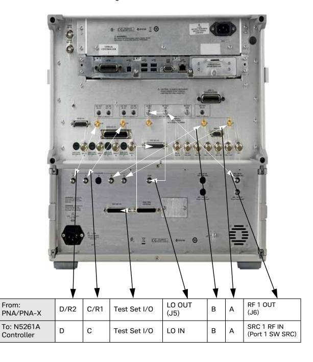
Figure 1-20 N5262A Rear Panel Configuration F
