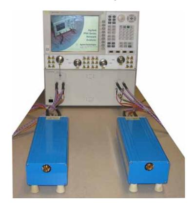
Figure 1-2 4-Port Banded Millimeter-wave Configuration (N5262A)
