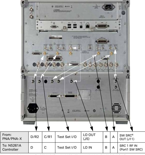
a. Install the adapter (N4903-61250) on the N5224/25A or N5244/45A SW SRC OUT (J11).
