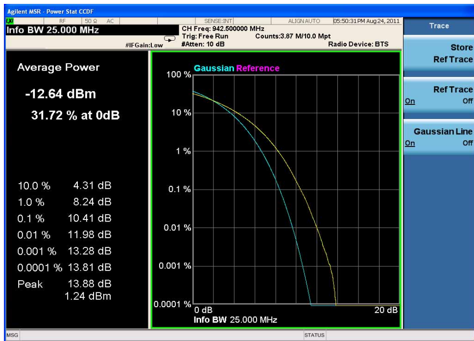
MSR Downlink Power Statistics CCDF Measurement Result
