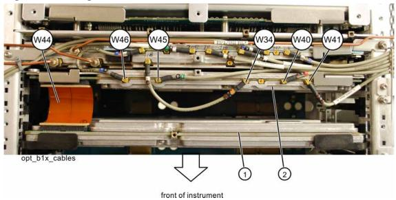
6. The Wideband Analog IF (2) and Wideband Digital IF (1) assemblies can now be removed by pulling up on the ejectors to remove from the chassis.
