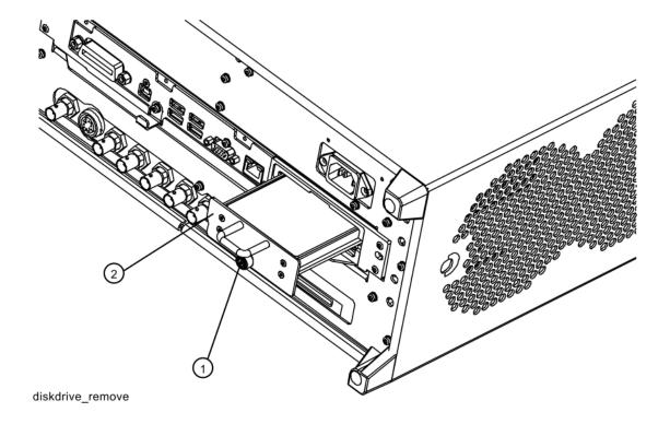
4. Refer to Figure 16-81. Remove the 4 machine screws (1) (0515-0372) from the disk drive carrier assembly that secure the drive (2).
