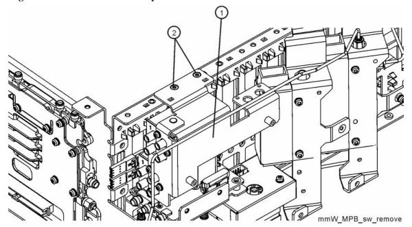
12. Refer to Figure 16-60. To separate the switches (2) and (4) from the bracket (1) (N9020-00021), remove the three screws (3) (0515-1934) for each switch.
