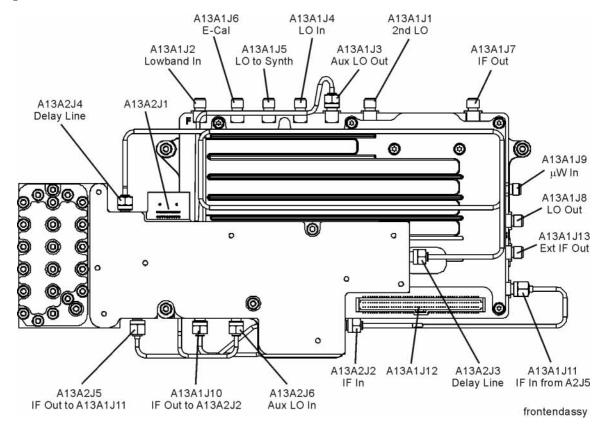
Expected signal is 4.8 GHz at  $-51 \text{ dBm} \pm 4 \text{ dB}$ . The tolerance is large because the A12 YTF (microwave preselector) loss varies between devices, and the YTF may not be perfectly aligned, or the frequency response adjustment may be required.
