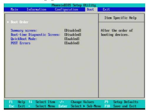
6. With Boot Order highlighted as shown in Figure 17-5 press Enter on the external keyboard to enter the Boot Order Configuration screen.
