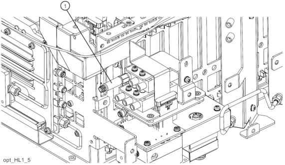
10. Refer to Figure 16-22. Disconnect the ribbon cable to the Front End Controller J802. Remove the switch assembly (1) by removing the two screws (0515-1035) at the frame (2) and the single screw on the side (3) (0515-0372).
