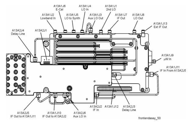
Expected signal is 4.8 GHz at  $-51 \text{ dBm} \pm 4 \text{ dB}$ . The tolerance is large because the A12 YTF (microwave preselector) loss varies between devices, and the YTF may not be perfectly aligned, or the frequency response adjustment may be required.
