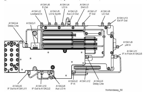
Connect A13J7 output to a functioning spectrum analyzer and verify the 322.5 MHz intermediate frequency is measuring  $-31 \pm 4$  dB as shown in Figure 5-5.
