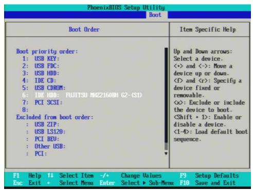
7. If IDE HDD is not listed first in the boot priority, press the Down Arrow on the external keyboard to highlight IDE HDD as shown in Figure 17-6.
