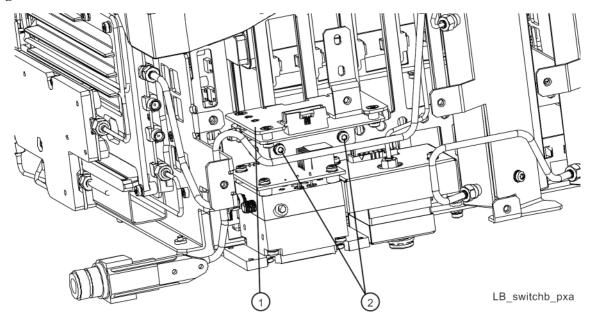
Figure 16-11 Low Band Switch and Bracket Separation
