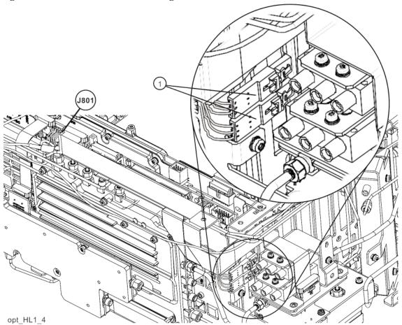
7. Refer to Figure 16-32. Attach the coaxial fixed attenuator (1) to switch port 1. Torque to 10 inch-lbs.
