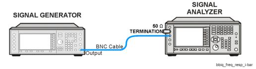
Figure 18-10 BBIQ Input Frequency Response Setup (Q Input)
