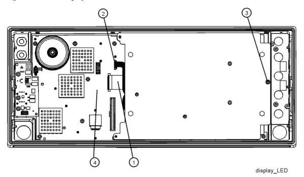
3. Remove the screw (3) (0515-0372) securing the display bracket to the Front Frame Assembly. The display can now be removed from the Front Frame Assembly.
