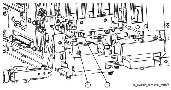
Figure 16-47 Low Band Switch and Bracket Separation
