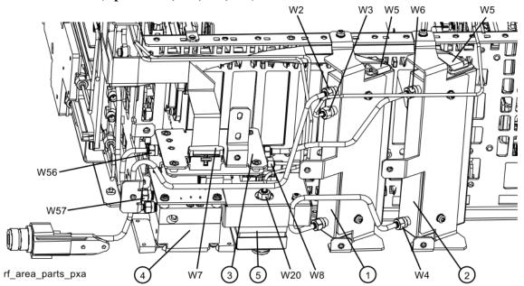
To gain access to the attenuators, low band switch, YTF Preselector, YTO, Option MPB, or Option LNP for removal, follow these steps:
