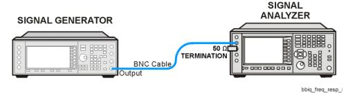
Figure 18-9 BBIQ Input Frequency Response Setup (I Input)
