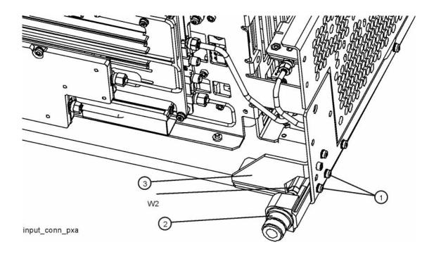
4. Remove the two screws (1) (0515-0372) that attach the Input Connector Assembly to the chassis. The connector assembly can now be lifted from the chassis.
