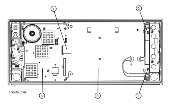
5. Remove the two screws (2) (0515-0372) securing the display bracket (3) to the Front Frame Assembly. The display can now be removed from the Front Frame Assembly.
