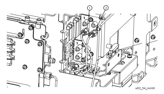
10. Refer to Figure 16-58. Disconnect the wire harness connector (1) located between the switch and the frame. Remove the ribbon cable from the rear of the top switch.
