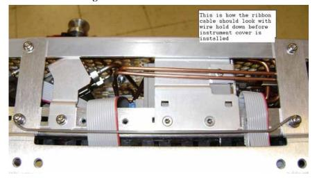
10. Refer to Figure 16-37. Install rigid cable W52 (N9020-20146) (1) between top switch port 4 and Low Band Switch Assembly connector that is closest to the inner chassis. Torque to 10 inch-lbs.
