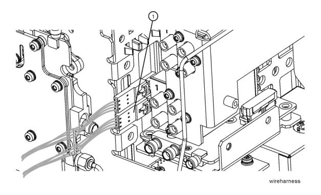
11. Refer to Figure 16-59. Remove the switch assembly (1) by removing the two screws (0515-1035) at the frame (2).
