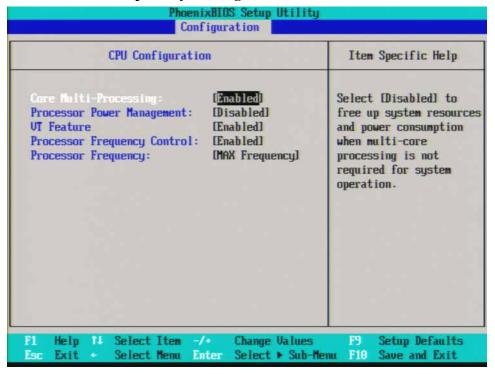
Figure 9-16 BIOS Setup Utility - Configuration > Advanced
