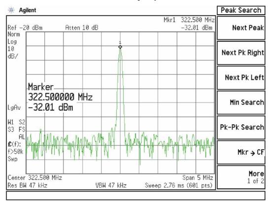
If this power level is correct the Front End assembly is operating correctly in high band. If this power level is incorrect verify the following assemblies using the 4.8 GHz internal calibrator signal.
