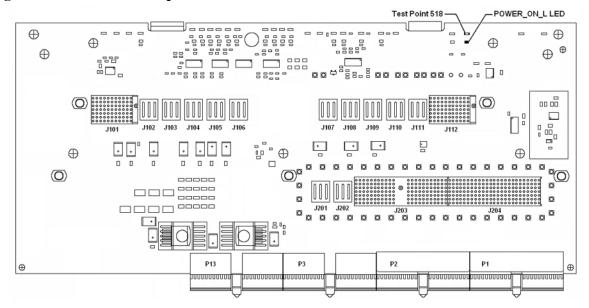
5. Turn the instrument power on from the front panel On/Off button and view the status of the POWER ON L LED, as shown in Figure 2-4.
