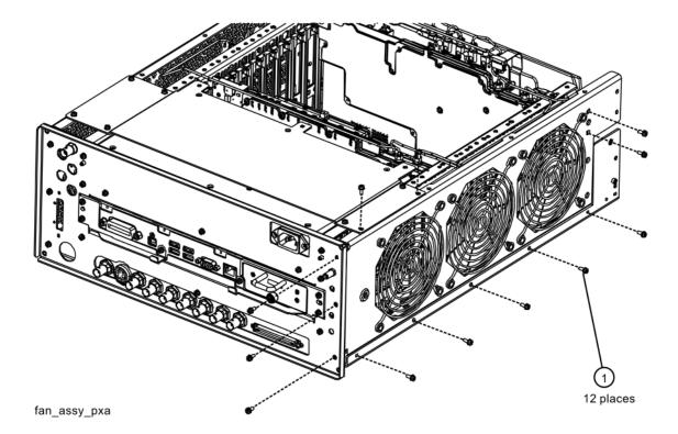
5. Refer to Figure 16-92. Unplug the fan wires from the motherboard. The fan assembly can now be lifted from the chassis.
