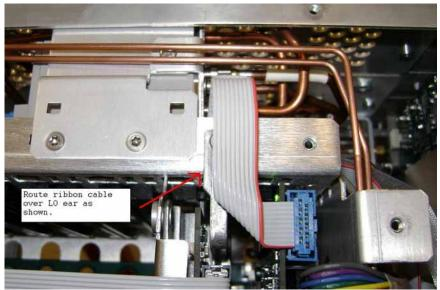
Figure 16-36 Cable Routing
