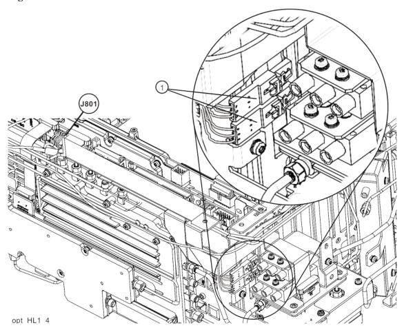
14. Refer to Figure 16-26. Remove the top switch/bracket assembly (1)/(2) by removing the single screw on the side (4) (0515-0372). To separate the switch from the bracket, remove the two top screws (3) (0515-0372).
