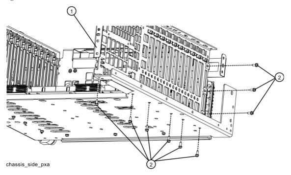
17. Refer to Figure 16-90. Remove the motherboard (1) by removing the four screws (2) (0515-0372). Slide the motherboard back off the standoffs and lift it up and out.
