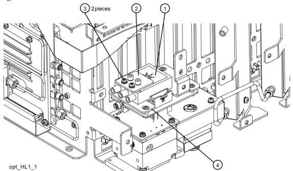
2. Refer to Figure 16-29. Place the second switch/bracket assembly (1)/(2) on the bracket previously installed. Assure Agilent label on switch is facing up. To attach use the two screws (3) (0515-1992).
