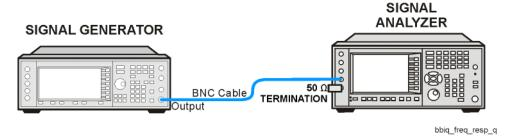
Figure 18-11 BBIQ Input Frequency Response Setup ( $\overline{Q}$  Input)
