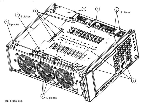
Figure 15-5 Top Brace and Reference Bracket
