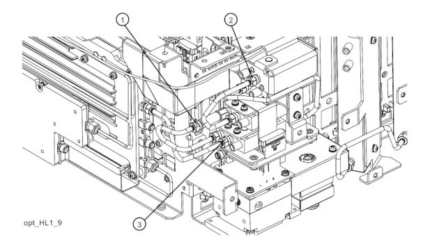
8. Refer to Figure 16-20. Remove cable W52 (N9020-20146) (1) between top switch port 4 and Low Band Switch Assembly connector that is closest to the inner chassis.
