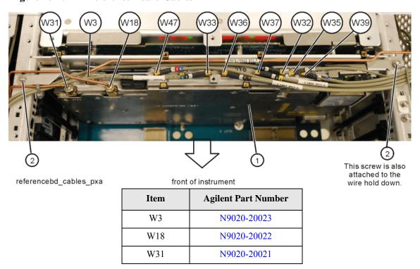
5. Remove the two screws (2) (0515-0372) attaching the Reference board to the chassis.
