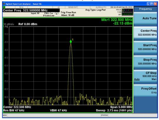
If this power level is correct the signal path from the A9 50 MHz Reference signal input port to A13A1J7, IF Output is operating correctly using a 50 MHz input calibrator signal. Reconnect the W16 cable to A13A1J7.
