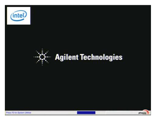
4. Press "F2" on the external keyboard when at the Agilent Technologies splash screen to enter the CPU BIOS Setup Utility as shown in Figure 17-4.
