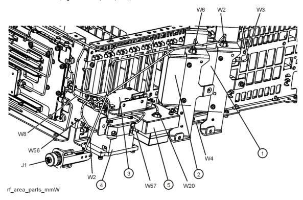
To gain access to the attenuators, low band switch, YTF Preselector, YTO, Option MPB, or Option LNP for removal, follow these steps:
