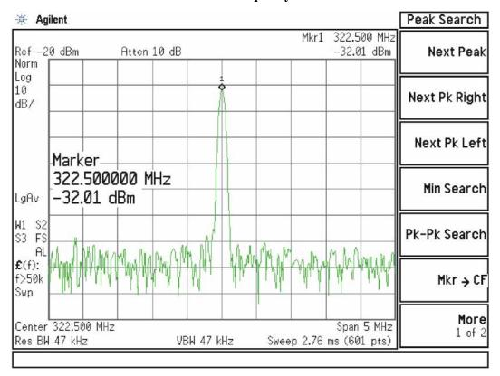
If this power level is correct the Front End assembly is operating correctly in high band. If this power level is incorrect verify the following assemblies using the 4.8 GHz internal calibrator signal.
