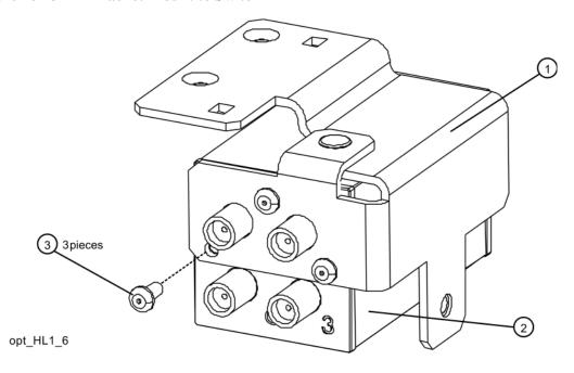
12. Refer to Figure 16-24. Disconnect W7 from the Low Band Switch.
