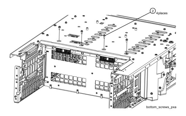
16. Refer to Figure 16-89. Remove the left side chassis (1) (same side as the fan) by removing the nine screws (2) (0515-0372) (six on the bottom).
