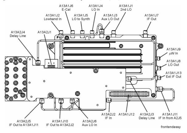
Connect A13J7 output to a functioning spectrum analyzer and verify the 322.5 MHz intermediate frequency is measuring  $-31 \pm 4$  dB as shown in Figure 4-5.
