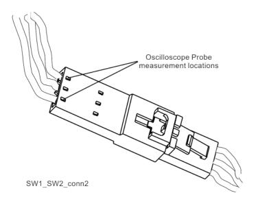
To verify the control logic, press **Mode Preset** on the analyzer. Press **FREQ**, **5 GHz**, **SPAN**, **1 MHz**, **AMPTD**, **More 1 of 2**, **uW Path Ctrl**. Standard Path is selected by default. Carefully place the scope probe tip on the conductive portion where the green wire goes into the connector, see Figure 6-8.
