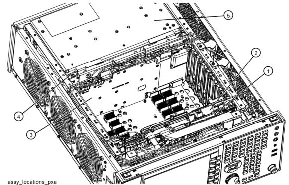
4. Refer to Figure 16-70. Remove cables W3, W18, and W31 from the reference assembly (1) using the 5/16-inch wrench.
