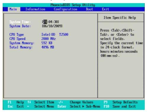
5. Press the Right Arrow on the external keyboard three times to highlight the Boot tab as shown in Figure 17-5.
