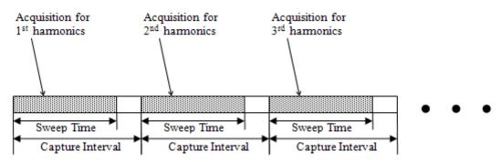
Sets the interval of capturing each harmonics. If the value is set to smaller than sweep time, it will be changed to the same value with sweep time.
