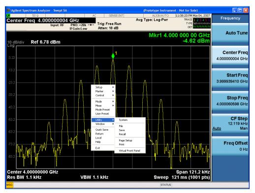
This method can be used to access any of the front-panel keys by using a mouse; as for example if you are accessing the instrument through Remote Desktop.
