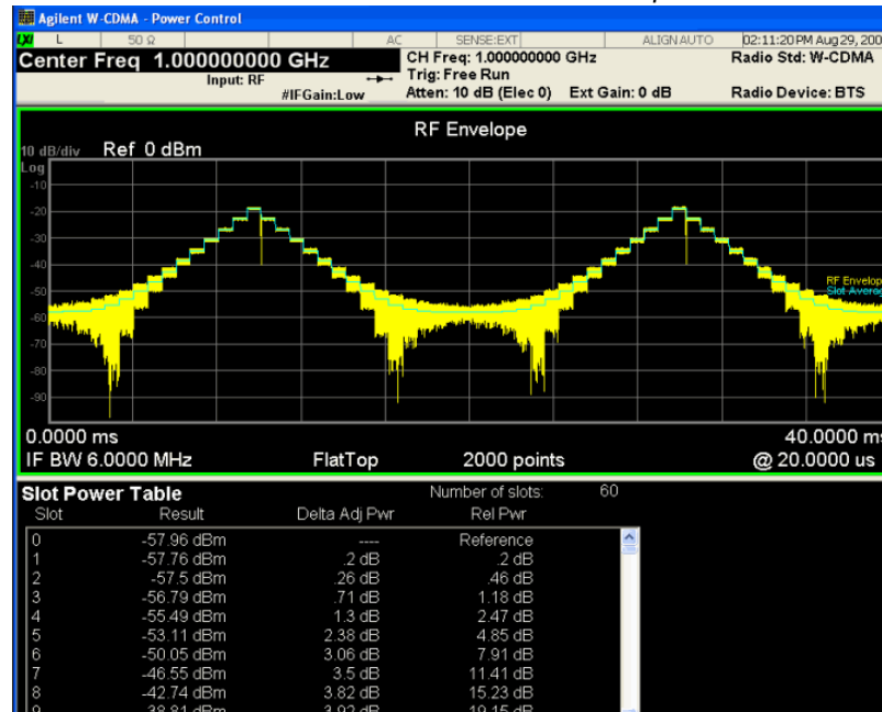
Power Control Measurement Result - Slot Power Graph Metrics View
