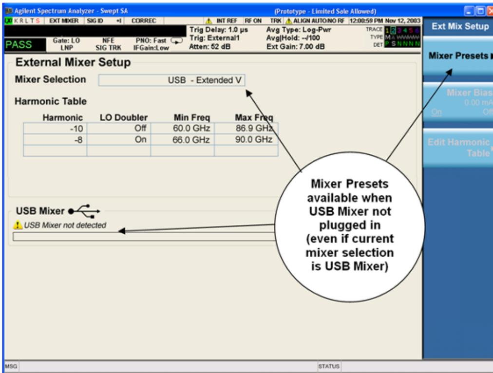
Only one USB Mixer is supported at a time. To switch to a different USB Mixer, disconnect the one that is no longer being used prior to connecting a new one.
