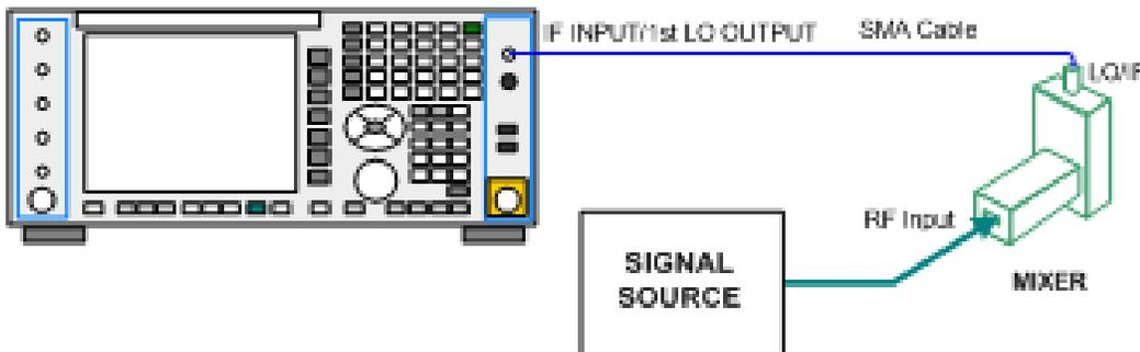
Legacy HP/Agilent and some third party mixers have separate LO In and IF out connections. This requires you to use an external diplexer to connect these mixers. A diplexer can easily be purchased for this purpose (for example, Diplexer Model # DPL.26 or # DPL.313B from OML Inc., Morgan Hill CA)
