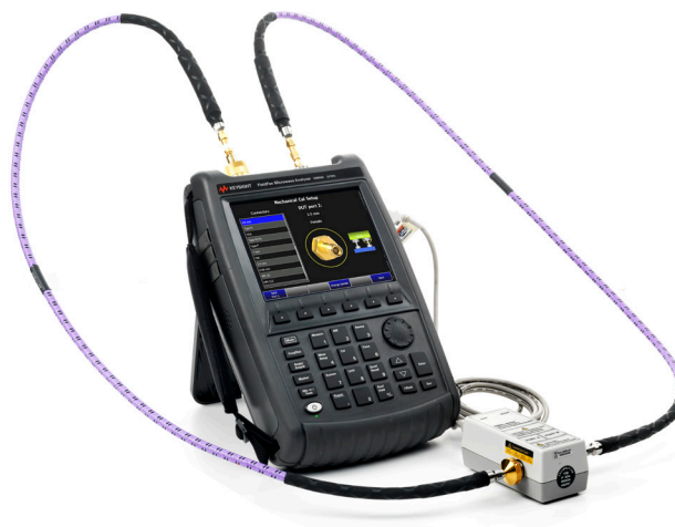
Keysight's value-line electronic calibration (ECal) modules make calibration of vector network analyzers fast, easy and accurate.
