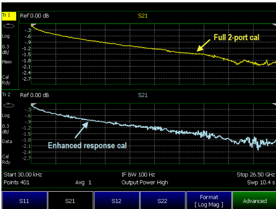
Figure 3. Measurement comparison of a coaxial cable using the FieldFox CalReady 2-Port calibration and the CalReady Enhanced Response calibration
