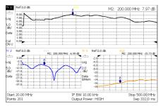
The above image shows a 3-trace configuration. **Tr1** is the **ACTIVE** trace as indicated by the highlighted **Tr1** annotation in the upper left corner.
