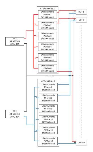
Power supply mux example 48 channels, 2 voltages
