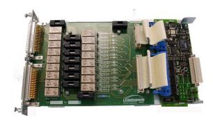
Figure 2. Keysight 34959A breadboard module with LXinstruments circuitry.
