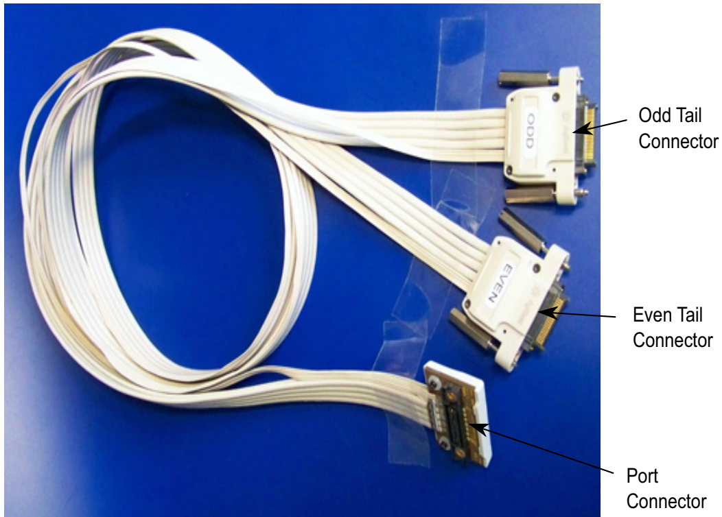
Figure 12 U4321-61601 Solid Slot Interposer Cable
