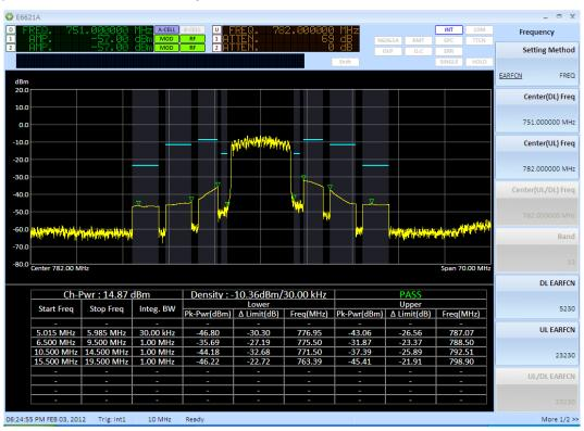
Figure 6-10: SEM measurement (FDD Example)
