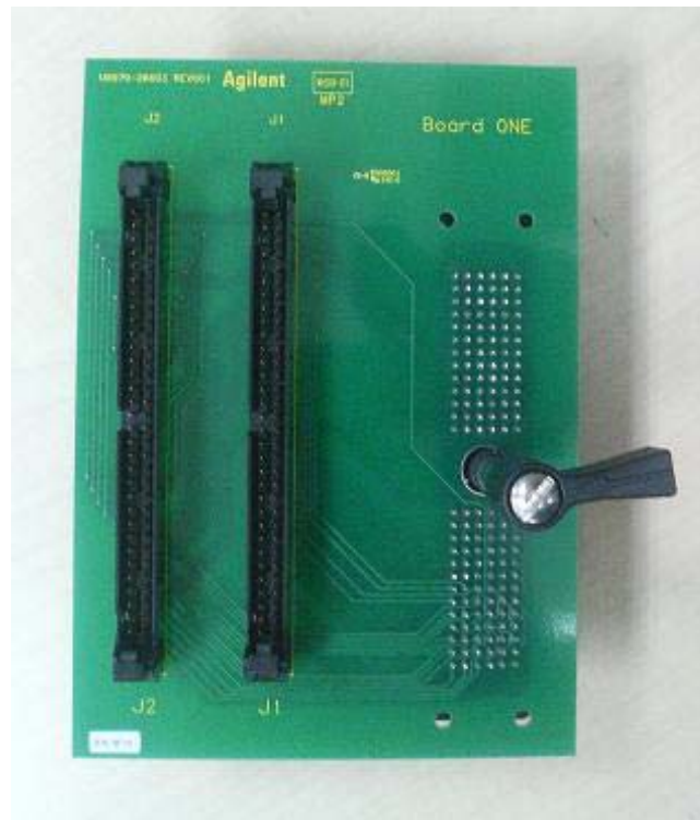
Figure 4-7 CEDGN Board #1 (U8970-66603 PCA- Diagnostic Number 1)
