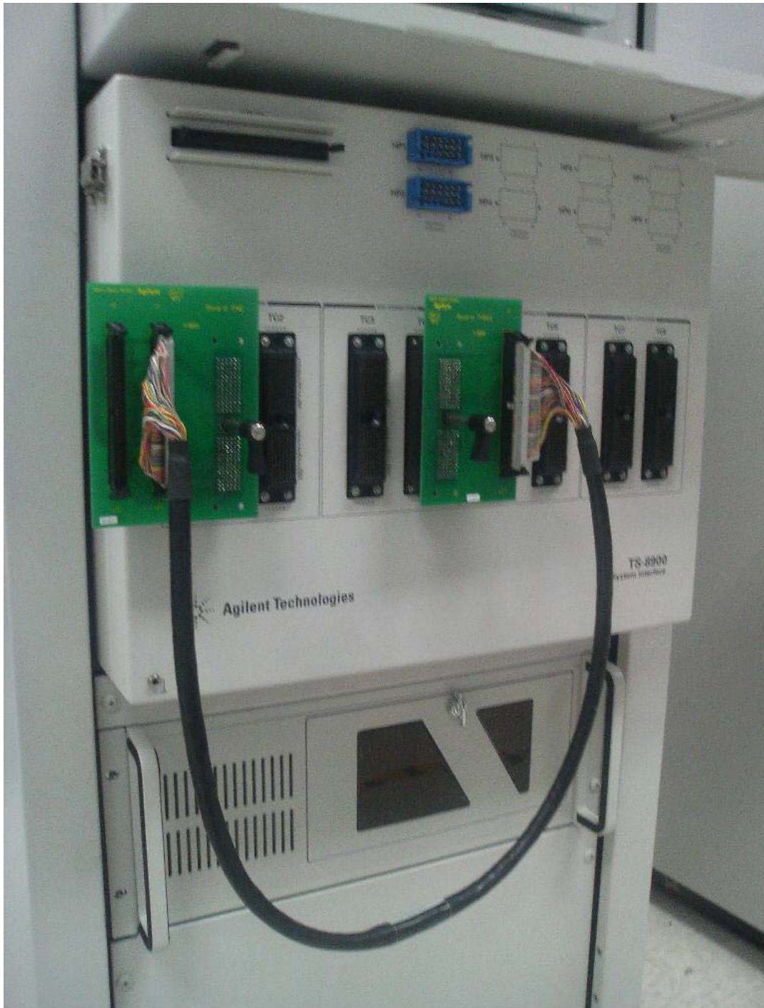
Figure 3-3 Installing CEDGN Board #1 (U8970-66603) to TC1 and CEDGN Board #3 (U8970-66605) to TC4 with both boards linked by cable (E6170-61607).
