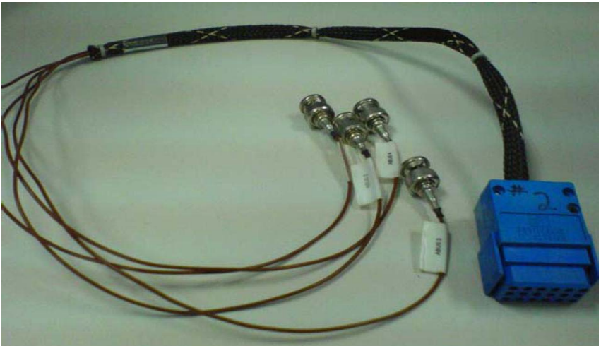
Figure 4-13 Diagnostic Cable (E6170-61618) for 8 Channel Heavy Duty Card
