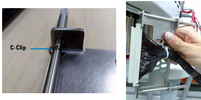
Figure 3-10 CEDGN Fixture Kit Bracket Installation Step 1
