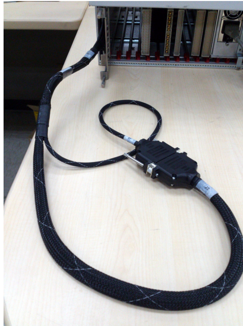
Figure 3-2 Installing the U8989-61625 CEDGN Test Fixture
