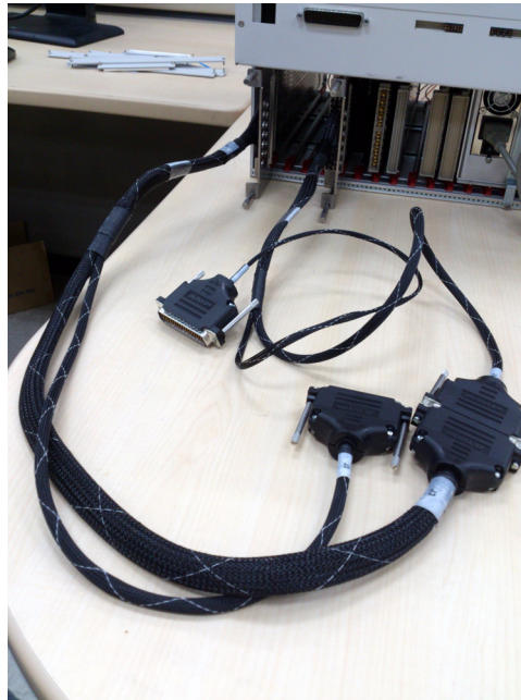
Figure 3-4 Installing the Load Card U8989-61 1 CEDGN Test Fixture with a U8989-61625CEDGN Pin Matrix Cable
