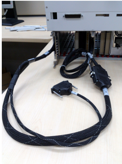
Figure 3-7 Installing the 48-Channel Load Card U8989-61622 CEDGN Test Fixture with a U8989-61625 CEDGN in Matrix Cable
