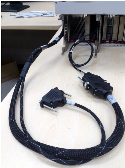
Figure 3-6 Installing the Heavy Duty Load Card U8989-61624 CEDGN Test Fixture with a U8989-61625 CEDGN Pin Matrix Cable
