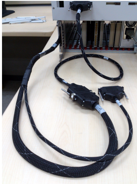
Figure 3-3 Installing the SLU Utility U8989-61620 CEDGN Test Fixture with a U8989-61625 CEDGN Pin Matrix Cable
