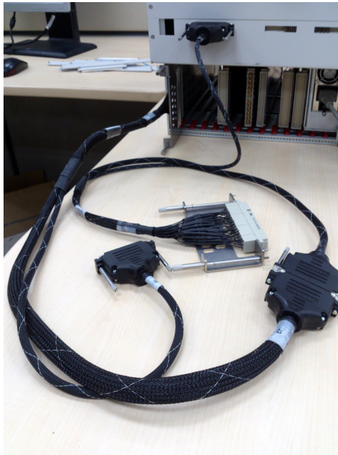
Figure 3-5 Installing the Load Card ISense U8989-61621 CEDGN Test Fixtures with a U8989-61625 CEDGN Pin Matrix Cable
