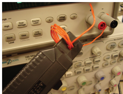
Figure 3. Improve the probe sensitivity by winding several turns of the conductor under test around the probe.
