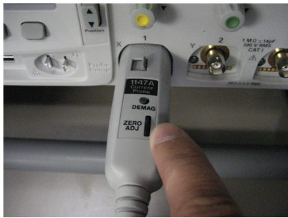
Figure 2. To improve current probe's accuracy remove magnetism and DC offset.
