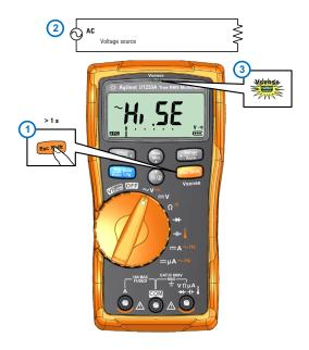
Press Range to change the Vsense detector's sensitivity from Hi.SE (high sensitivity) to Lo.SE (low sensitivity).
