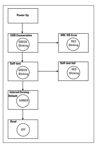
Figure 1-1 LED indicator sequence during power-up
