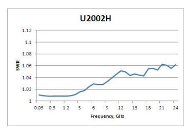
**Figure 3-7** U2002H Typical SWR (25 °C  $\pm$ 10 °C)
