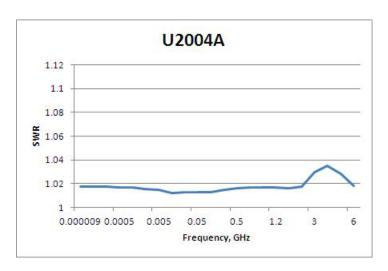
**Figure 3-4** U2004A Typical SWR (25 °C  $\pm$ 10 °C)
