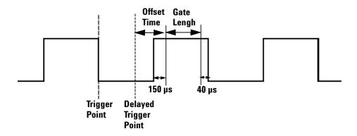
Figure 2-2 Measurement gate
