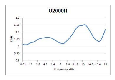
**Figure 3-5** U2000H Typical SWR (25 °C  $\pm$ 10 °C)
