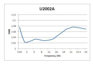
**Figure 3-3** U2002A Typical SWR (25 °C  $\pm$ 10 °C)
