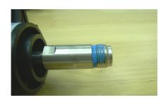
**1** Apply one drop of loctite on the first, second, and third threads of the connector.
