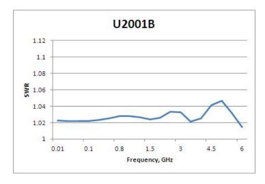
**Figure 3-9** U2001B typical SWR (25 °C  $\pm$ 10 °C)
