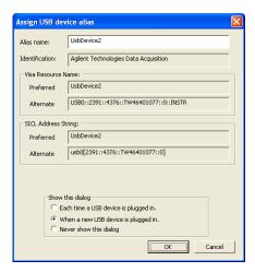
Figure 1-8 USB device alias configuration
