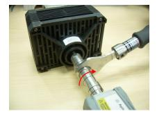
**2** Tighten the connector using the torque wrench.
