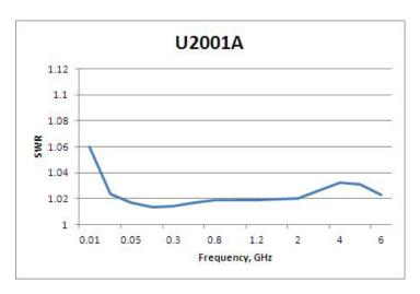
**Figure 3-2** U2001A Typical SWR (25 °C  $\pm$ 10 °C)
