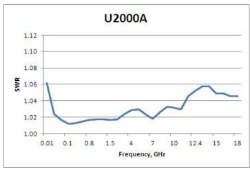
**Figure 3-1** U2000A typical SWR (25 °C  $\pm$ 10 °C)
