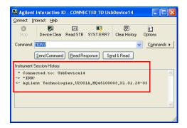
Figure 1-11 Identification of your connected power sensor displayed
