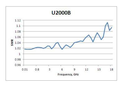
Figure 3-8 U2000B typical SWR ( $25 \, ^{\circ}\text{C} \pm 10 \, ^{\circ}\text{C}$ )
