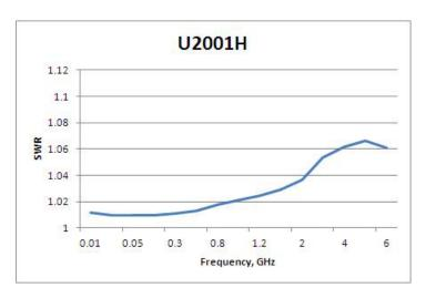
**Figure 3-6** U2001H Typical SWR (25 °C  $\pm$ 10 °C)
