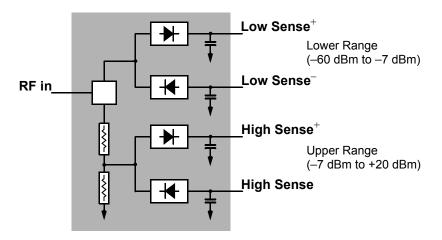
Figure 1-3 Simplified block diagram of diode pair/attenuator/diode pair
