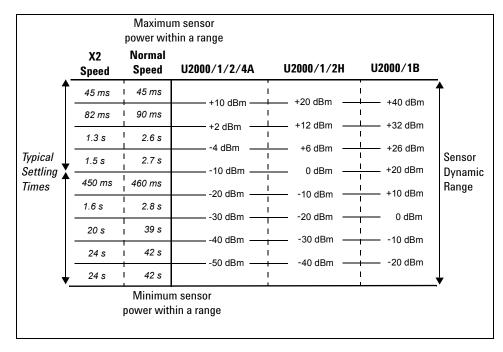
Figure 3-13 Settling time with auto filter, default resolution, and a 10 dB decreasing power step (not across the switching point)
