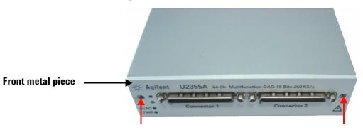
Step 5: Gently pull the front metal piece out, which is attached to the carrier and measurement boards.
