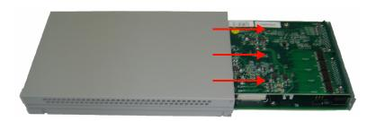
Step 6: Unscrew all the following indicated screws from the metal casing and remove the rear metal piece.
