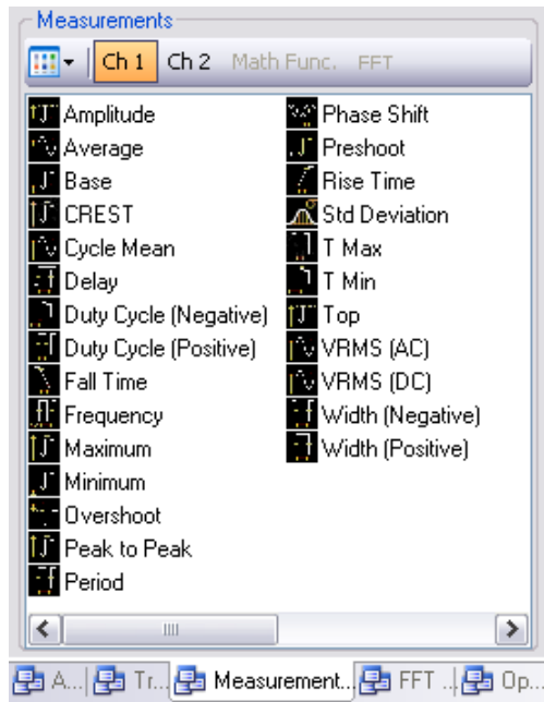
Figure 2-8 Automatic measurements on the Measurements & Cursors panel
