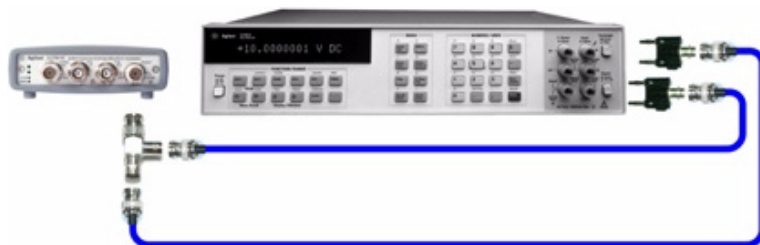
Figure 3-2 U2761A to DMM four-wire connection
