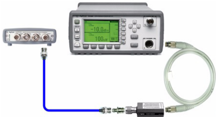
Figure 3-4 U2761A to power meter connection
