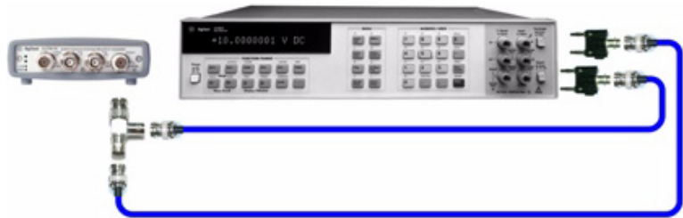
Figure 3-5 U2761A to DMM four-wire connection
