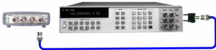
Figure 3-3 U2761A to DMM connection
