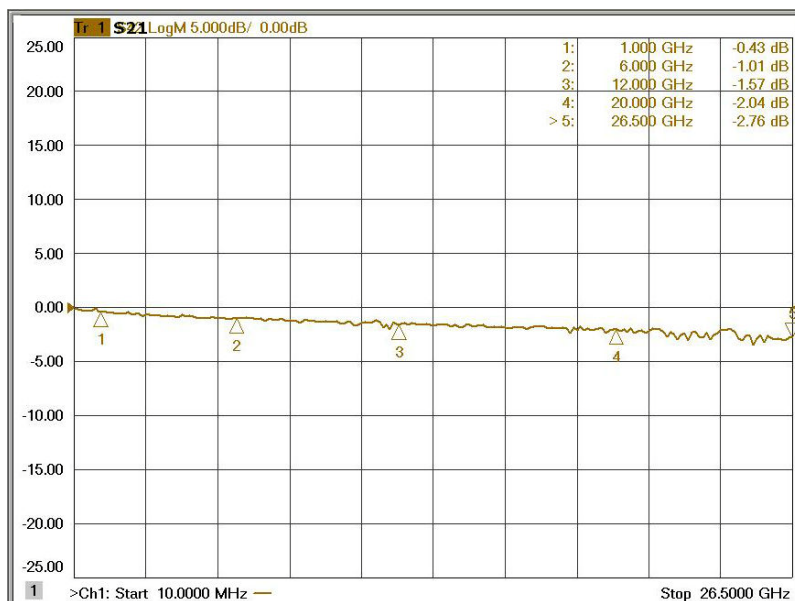
Figure 9 Typical S21 Response Plot
