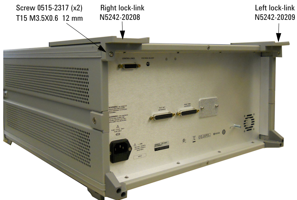
Figure 8 Install Lock-links to the Test Set
