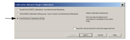
4. Continue following the Cal Wizard prompts. In the "Select Calibration Ports and ECal Module" dialog box press Select All, or select the ports you are calibrating and press Next. If an ECal characterization has been done, select View/Select ECal Module and select the previously saved user file from step 3.
