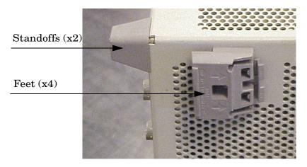
4. Install the two rear locking feet (5023-0132) onto the PNA or PNA-X, where the standoffs were removed.
