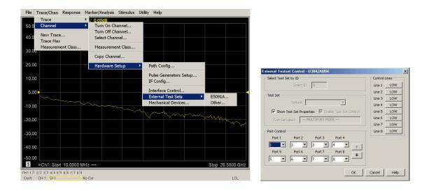
This menu will allow the physical Ports 1 thru 8 to be identified as any port for your convenience. For example; Port 5 can be re-named Port 2.
