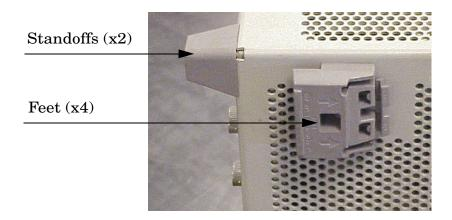
4. Install the two rear locking feet (5023-0132) onto the PNA-L, where the standoffs were removed.
