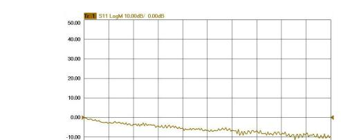
Figure 19 Typical Reflection Response Ports 1-4
