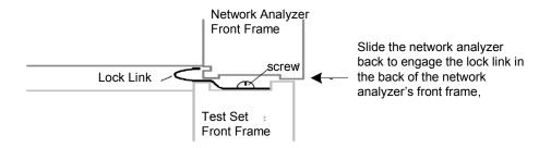
Figure 10 Locking Feet Screws
