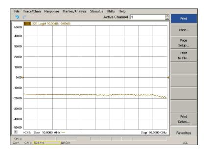
Connect the RF Flex cables to the Source IN and CPLR THRU port indicated in Table 20 and Table 21, the expected results should be similar to Figure 53.
