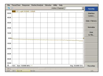
Connect the RF Flex cables to the Test Port and RCVR OUT port indicated in Table 19. The expected results should be similar to Figure 52.
