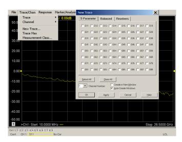
Figure 26 New S-Parameter Measurement
