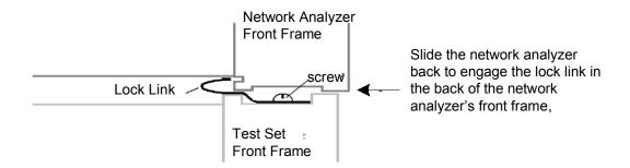
Figure 16 Locking Feet Screws
