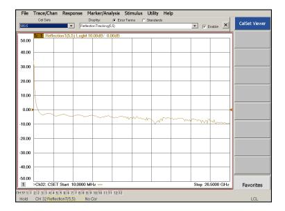
Figure 45 Reflection Tracking Trace (Port 5-8) with PNA or PNA-X
