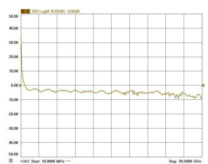
Figure 21 Typical Reflection Response Ports 5-8
