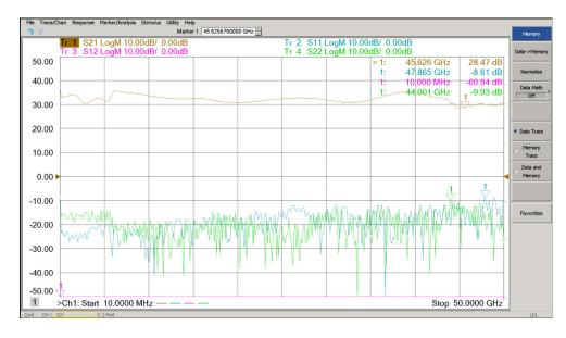
Figure 17 Typical Option 050 Port12 S-Par Plot
