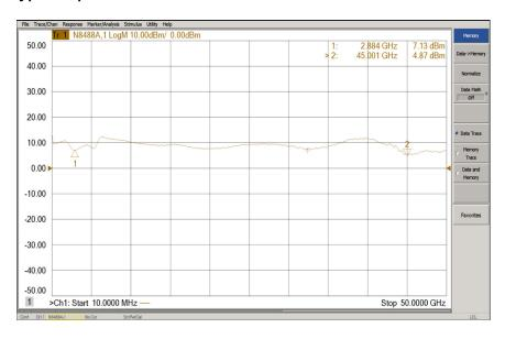
Figure 19 Typical Option 067 Port21 S-Parameter Plot
