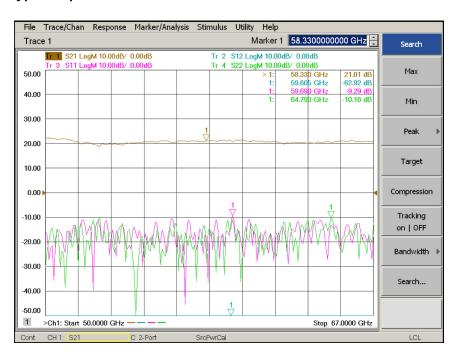
Figure 20 Typical Option 067 Port12 S-Parameter Plot
