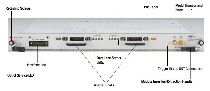
Figure 1 U4431 Module Components
