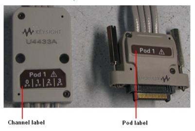
Figure 11 U4433 Channel Label and Pod Label
