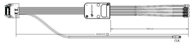
Figure 5 U4433A Probe Dimensions
