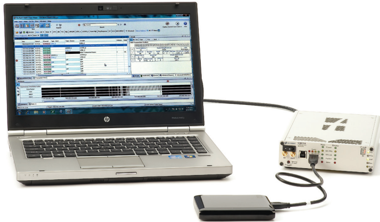
Figure 1. The U4611A/B Analyzer is connected in a pass-through mode and records traffic being exchanged between the host and the device under test.
