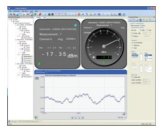
The bundled N1918A Power Panel software offers multiple display types for convenient power measurement and analysis.
