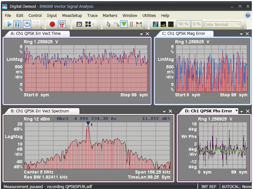
Figure 24. Trace A, error vector time, shows the error vector magnitude at the symbol points. Trace B, error vector spectrum, shows the frequency spectrum of the error vector time data. Trace C, IQ mag error, is the magnitude difference between the measured and reference IQ waveforms. Trace D, IQ phase error, is the phase difference between the measured and reference IQ waveforms.
