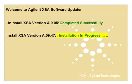
The new instrument software is being installed. The "Installation in Progress" text will roll across the screen indicating software activity. There will be several windows appearing and disappearing during this time. NO interaction with the instrument is required. Please be patient the total software installation process can take 35 to 40 minutes. It will display "Completed Successfully" when the software update is complete. You will be prompted to restart you instrument at the end.
