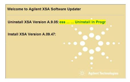
The old instrument software is being removed. The "Uninstall in Progress" text will roll across the screen indicating software activity. There will be several windows appearing and disappearing. It will display "Completed Successfully" when this step is finished.
